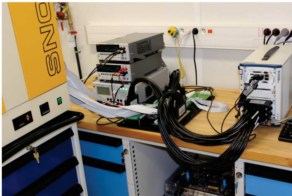
FIGURE 3.19 – Banc de test High Temperature Gate Bias (HTGB)
