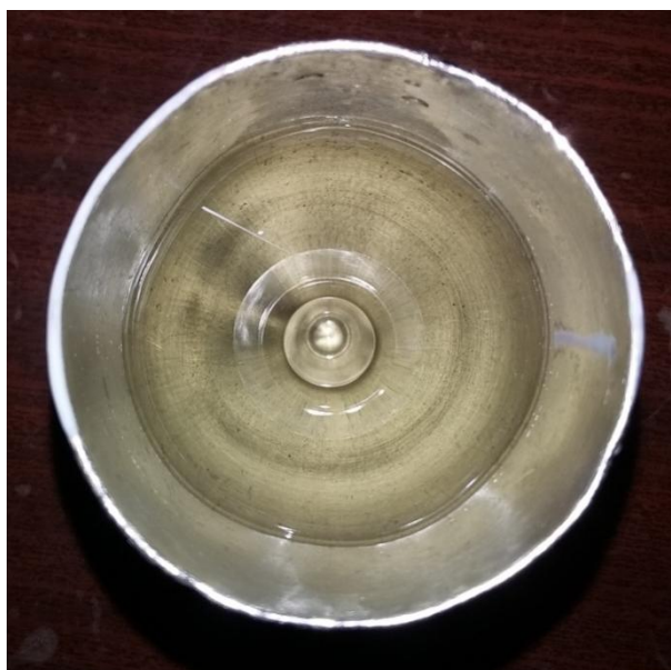
Figure 2.6 Crucible with the solution melt used for synthesizing \text{GaBO}_3 crystals after extracting from the muffle furnace.
