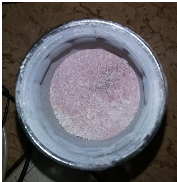
Figure 2.5 Prepared charge used in synthesizing \text{Fe}_x\text{Ga}_{1-x}\text{BO}_3 crystals of a definite composition.
