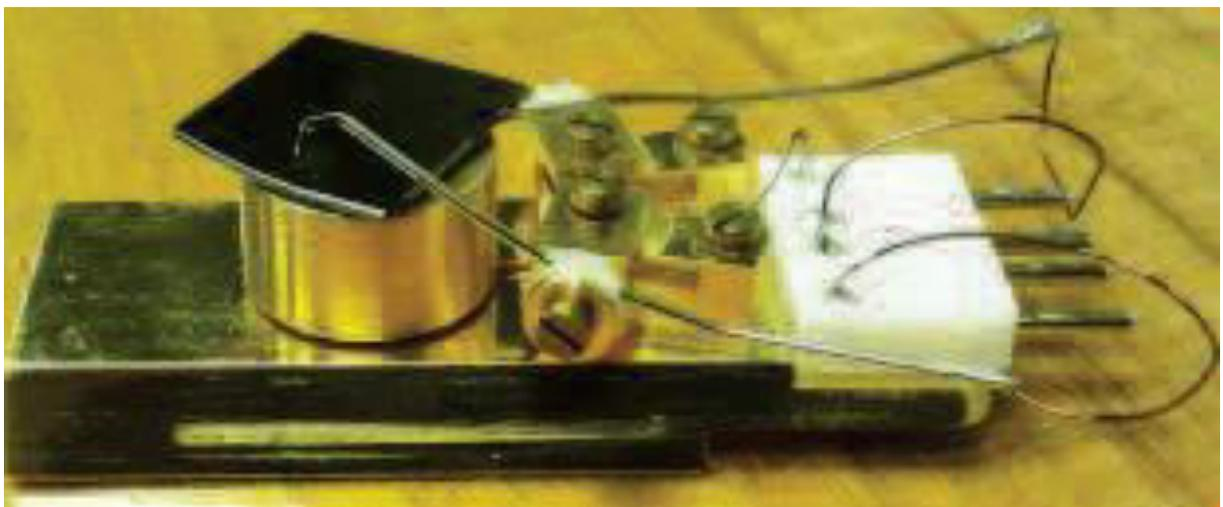
Figure E.4: Advanced EBIC sample holder with two probes.
