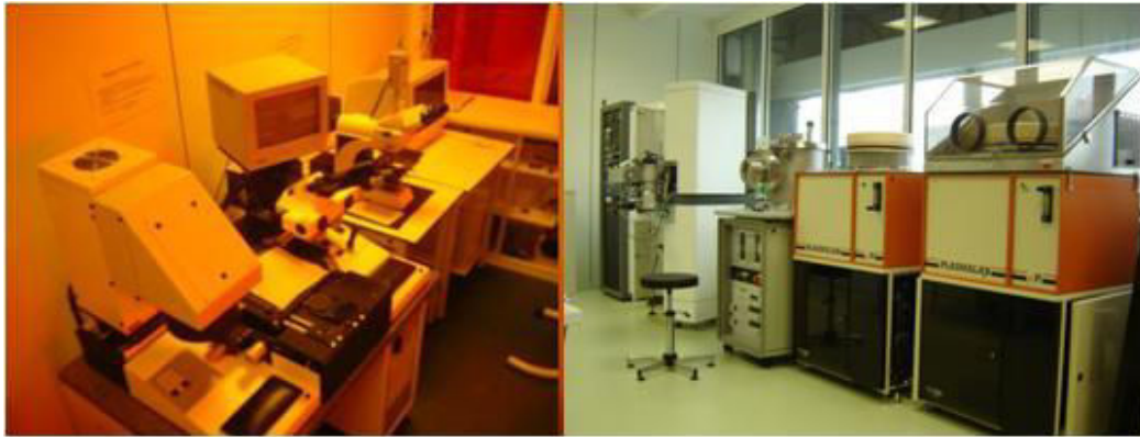
Figure D.4: Minalor clean-room facilities and equipment's used in our device processing and fabrication. To the right is the "salle rouge" for doing lithography and to the left is the sputtering and thermal evaporator for doing metal deposition.
