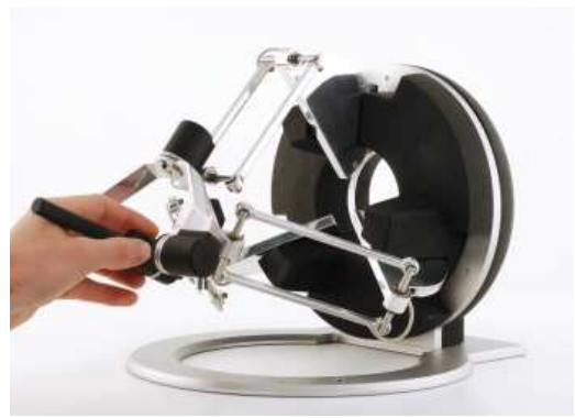
Figure 1.17 – Omega.6: a 6-DOF parallel haptic device
