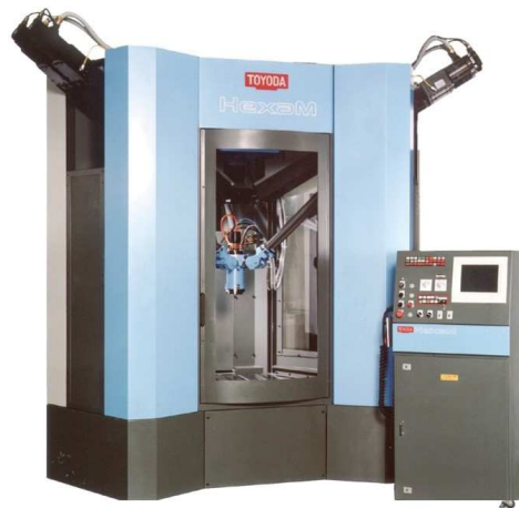
Figure 1.11 – Toyota HexaM PKM-based machine tool (US Patent 5,715,729) [Toyama et al., 1995]
