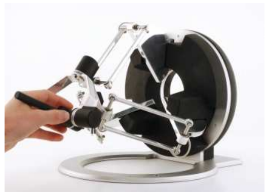
Figure 1.17 – Omega.6: a 6-DOF parallel haptic device
