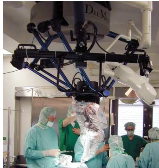
(b) SurgiScope: a Delta robot carrying a microscope (Elekta)
