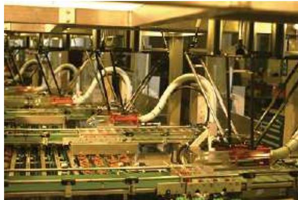
Figure 1.13 – Industrial bakery powered by parallel robots
