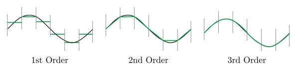
Figure 3.3: Reconstruction (green) of the initial function (black) with a first (left), second (middle), and third (right) order scheme.
