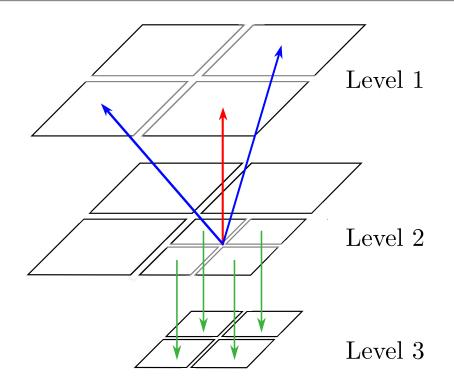
Figure 3.5: 2D representation of the oct-tree structure of RAMSES. Each oct (here on Level 2) points to it's mother cell (red arrow) and the neighbouring mother cells (blue arrows), and to it's children octs (green arrows).
