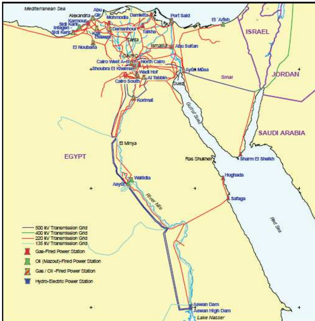
Figure 2-7: Electricity generation and transmission infrastructure in Egypt in 2010
