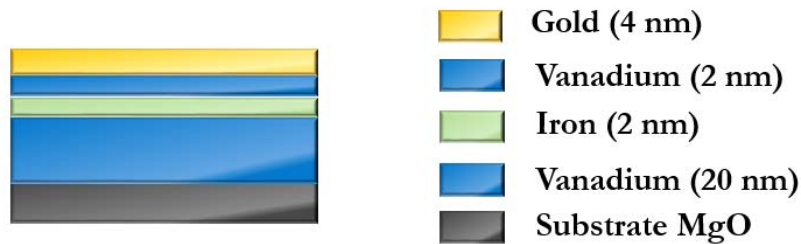
Figure 3-7_ Sample composition (applicable to all the samples used for the realization of artificial spins systems in this work). The mentioned thicknesses are the nominal thicknesses, and so the effective thickness of Iron is 1.7 nm.
