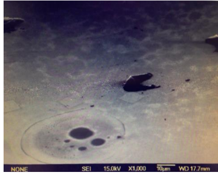
Figure 3-11_ MEB image after chemical etching of the aluminum layer. The surface appears dirty due to the attack of the remover on the Vanadium layer.
