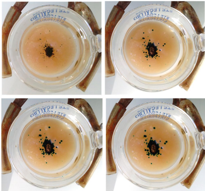
Figure 54: Methylene blue expansion in apple purée at 80°C as a function of time.
