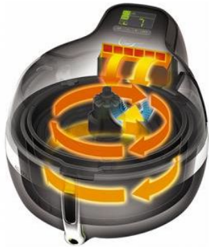
Figure 27: Principle of heat treatments by Actifry ® devices.
