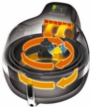
Figure 27: Principle of heat treatments by Actifry ® devices.
