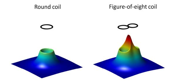
**Figure 1.4** Shape of stimulation coils and their associated magnetic field. Classic round shaped coil with its associated magnetic field, showing strongest field intensities under the edges of the coil. A figure of eight coil with it associated magnetic field, with strongest field intensities under the central intersection of the two adjacent coil loops.
