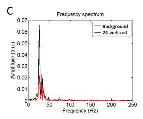
**Figure D.1** Vibration measurements of the 24 well coil (A, red) and background surface (B, black) in mm/s as measured by a single point vibrometer with OFV-534 compact sensor head for high optical sensitivity. Vibration velocity of coil is below background vibration. C) Fourier transform of the frequency spectrum, confirming below background amplitude vibrations as shown in Chapter 2/article for publication).
