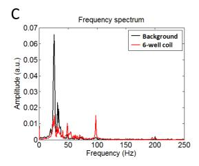
**Figure D.2** Vibration measurement of the 6 well coil (A, blue) and background surface (B, black) in mm/s as measured by a single point vibrometer with OFV-534 compact sensor head for high optical sensitivity. Vibration velocity of coil is below background vibration. C) Fourier transform of the frequency spectrum confirming total below background amplitude vibrations.
