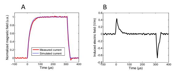
**Figure 3.7** A) Single pulse waveform in normalized, arbitrary units (a.u.). Intensity inside the coil modelled in Tina (blue dotted line) and magnetic field strength measured via hall effect (red line), showing a tight correspondence between predicted and measured waveform. B) Calculated, single pulse induced electric field in a round conductor at a radius of 2 mm from the central axis and 4 mm vertically above the top of the coil's wiring.
