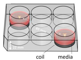
**Figure 4.4** Culture set-up and pulse delivery. Number of pulses delivered per 10 min stimulation session (A) and schematic view of *in vitro* culture set-up for stimulation (B). B) Coils were centered below the well of a 6 well plate resulting in 4 mm distance from the centre plane of the explant located on the Millicell membrane.
