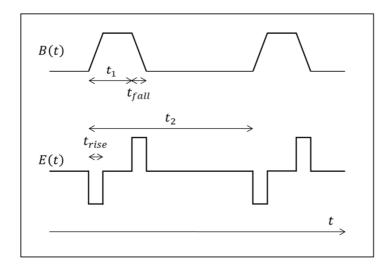
Figure 3.2 Desired magnetic field (B(t)) and the predicted induced electric field inside a conductor (E(t)). Three different temporal domains are specified for this set-up:  $t_{rise}$  = rise-time,  $t_{fall}$ = fall-time , $t_1$  = pulse ON and  $t_2$  = inter-pulse interval (frequency).  $t_{rise}/t_{down}$  and  $t_1$  are based on previous experiments and have a value of 100  $\mu$ s and 300  $\mu$ s respectively;  $t_2$  is experiment dependent.
