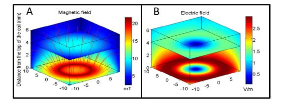
**Figure 3.6** A) Modelled overview of magnetic field strength (mT; colours) and direction *B* (red lines) starting at the top of the coil wiring (horizontal plane at 0 mm). B) Modelled overview of the induced electric field from the top of the coil wiring (Horizontal plane at 0 mm). Colours indicate the electric field strength (V/m). A,B: Horizontal plane at 4 mm corresponds to target tissue location.
