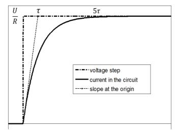
**Figure 3.4** Definition of the characteristic time Tau ( $\tau$ ). Current intensity inside the circuit in response to increasing voltage steps reaches more than 99.9% of its maximum after a time of  $^{\sim}5\tau$ .
