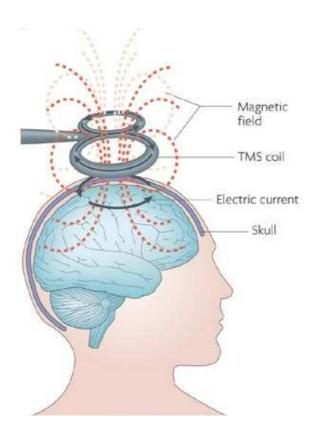
Figure 1.1 Overview of electromagnetic induction in TMS. A pulsed (time varying) primary current inside the coil creates a changing (time varying) magnetic field. Which induces an electric field, that creates a secondary electric current in conductive brain tissue in an opposite direction to the primary current. Image adapted from Ridding & Rothwell (2007).
