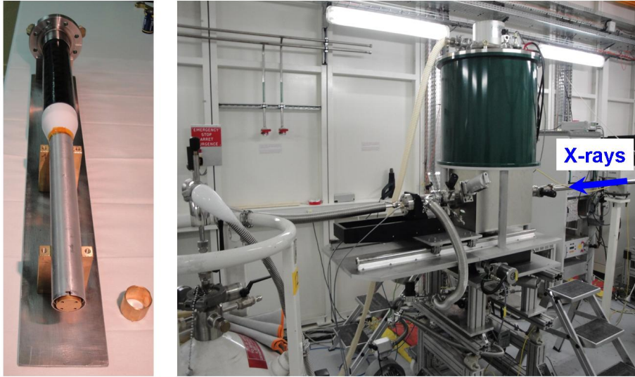
Figure 2.7 Probe (left) and the fridge with the X-rays line (right) used at the ID12 line at ESRF. Courtesy of F. Wilhelm and A. Rogalev.
