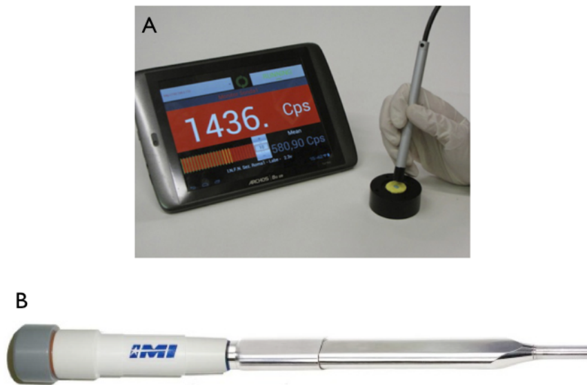
Figure 1.8 – Image of the intraoperative \beta counting probe developed by Camillocci et al. with a screen to display in real-time the counting rates (A) and image of the wireless Beta Probe from IntraMedical Imaging (B).
