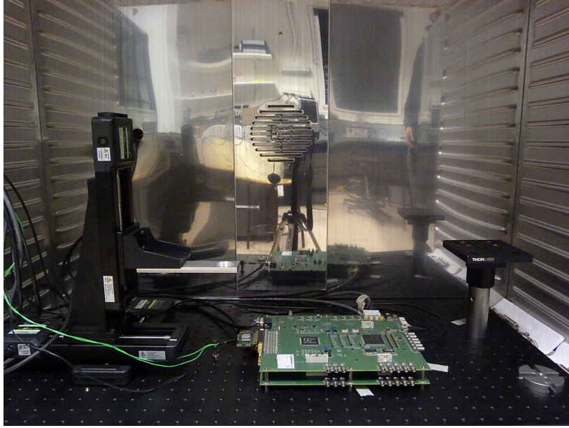
Figure 3.1 – Photography of the experimental set-up: 3-axis motorized platform and the EASIROC board inside the climatic chamber.
