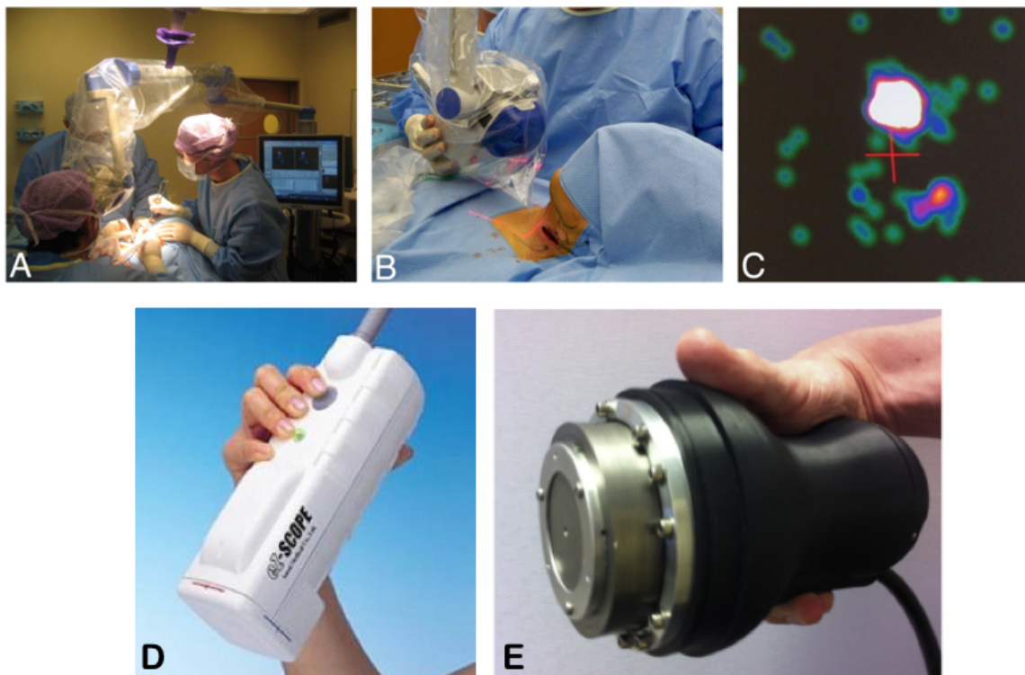
Figure 1.7 – Surgeon positioning the sterile-wrapped head of the \gamma -camera Sentinella ® (S102, Oncovision) using a laser pointer (A,B) and the relative image of a sentinel lymph node (C). Miniaturized portable gamma cameras eZ-scope ® (Anzai) (D) and Compact Gamma Camera (CGC) from Bugby et al. (E).
