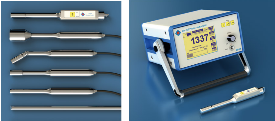
Figure 1.6 – (Left) From the bottom to the top gamma counting probes for laparoscopic use and a shorter version, high sensitivity probe, articulatable hand held probe, probe dedicated to the detection of high energy gamma rays produced by positron emitters and wireless probe. (Right) Wireless gamma counting probe with its Bluetooth connected control module (manufactured by Crystal Photonics Germany) [CrystalPhotonicsGermany 2016].
