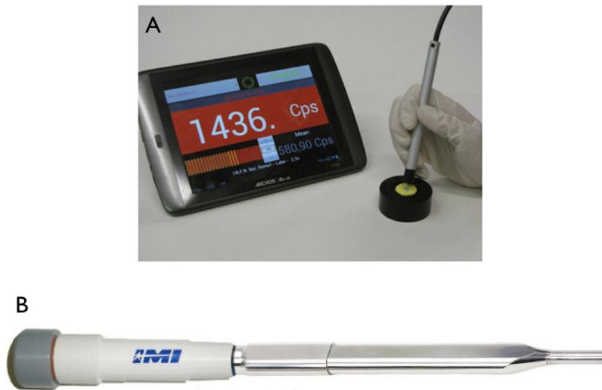
Figure 1.8 – Image of the intraoperative  $\beta$  counting probe developed by Camillocci *et al.* with a screen to display in real-time the counting rates (A) and image of the wireless Beta Probe from IntraMedical Imaging (B).
