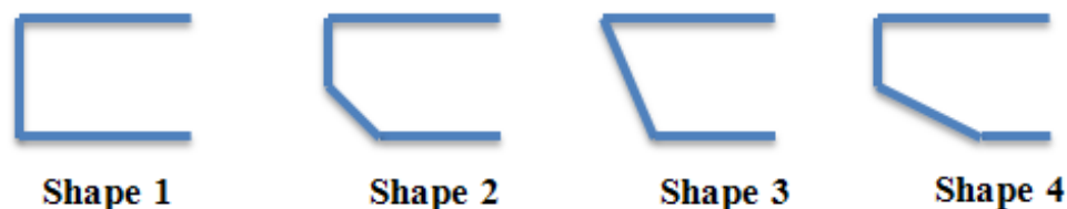
Fig. 2.12 : Different shapes of magnet due to optimizing process against demagnetization fault [31] (Finally, the author Introduces the shape model 1 as a robust permanent magnet type of outer rotor PMSM for HEV)
