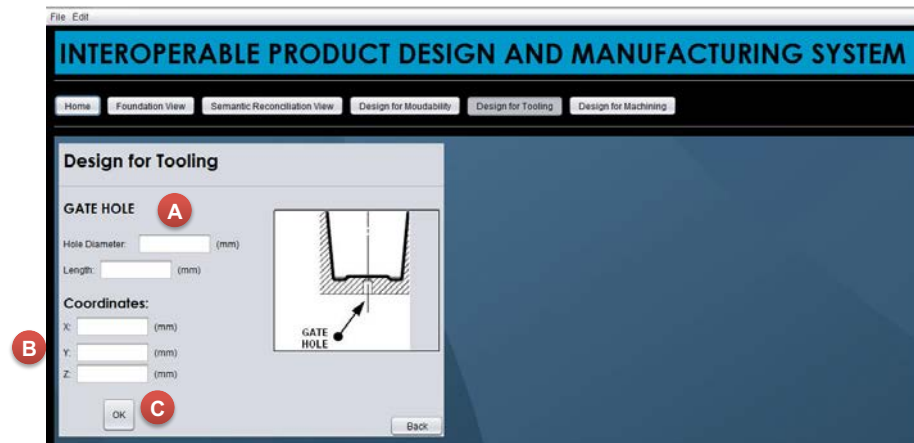
Figure 143 Gate hole interface in the IPDMS.
