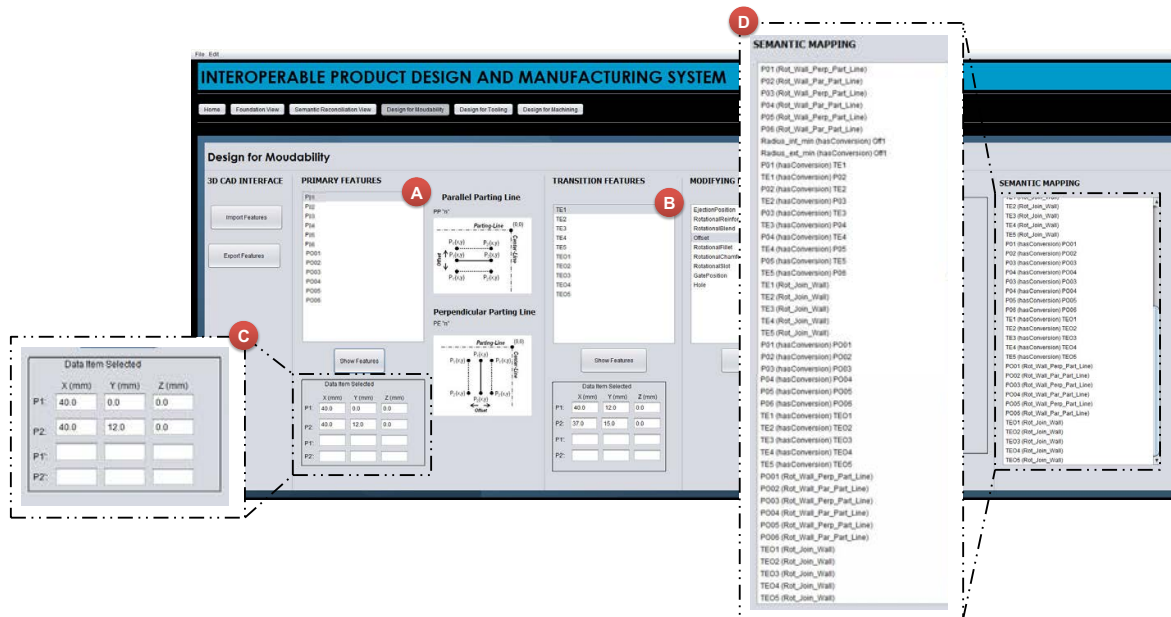
Figure 151 Design for Mouldability interface in the IPDMS with the transition features and the offset features.
