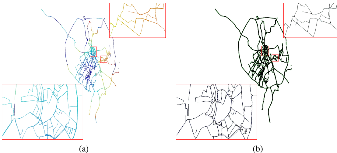
Figure 3.16: GPS data - (a) The distance functions d on each connected components. The value increases from cold to warm colors. (b) The reconstructed \alpha -Reeb graph.
