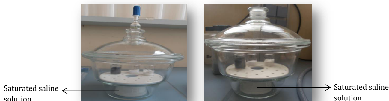
Figure 2-16. The storage conditioning setups of the aging experiments without the air passage (left) and with the air ( \text{CO}_2 ) passage (right)
