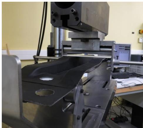
(b) Rupture de la mini-structure
