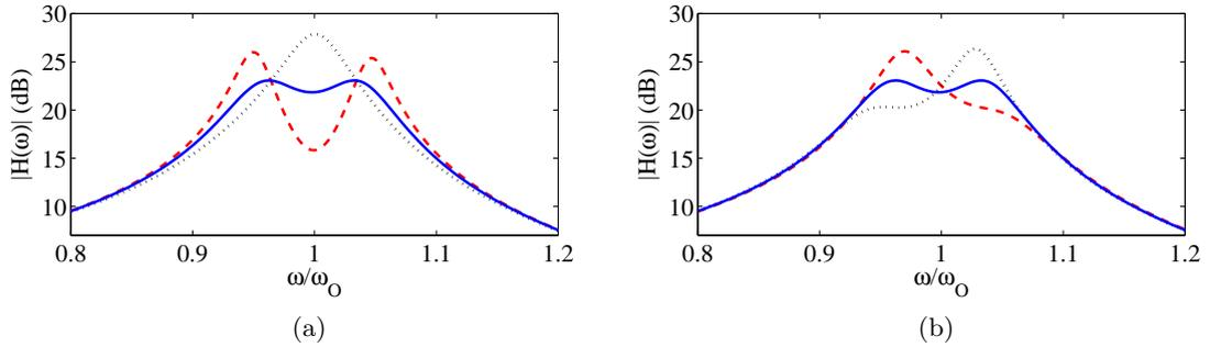
Figure 2.7: Modulus of the transfer function  $H(\omega)$ : (a) Tuning of the resistance - ( $-$ ) with the optimal resistance, ( $\cdots$ ) with twice the optimal resistance, ( $-\cdot-$ ) with half of the optimal resistance. (b) Tuning of the inductance - ( $-$ ) with the optimal inductance, ( $\cdots$ ) with 105% of the optimal inductance, ( $-\cdot-$ ) with 95% of the optimal inductance.
