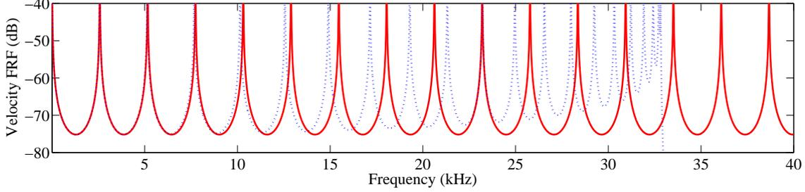
Figure 3.5: Velocity FRFs - (—) for the continuous rod, ( $\cdots$ ) for the lattice model.
