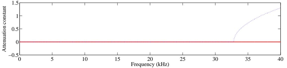
Figure 3.3: Attenuation constants - (—) for the continuous rod, (···) for the lattice model.
