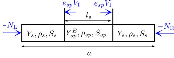
Figure 3.18: Piecewise homogenized model for the rod segment.
