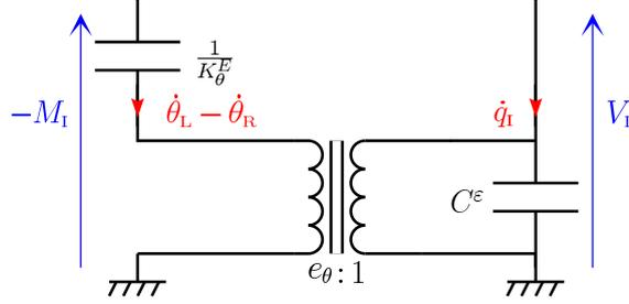
Figure 4.8: Model of the piezoelectric coupling for a unit cell subjected to bending.
