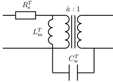
Figure 4.23: Simplified equivalent circuit of a non-ideal transformer.
