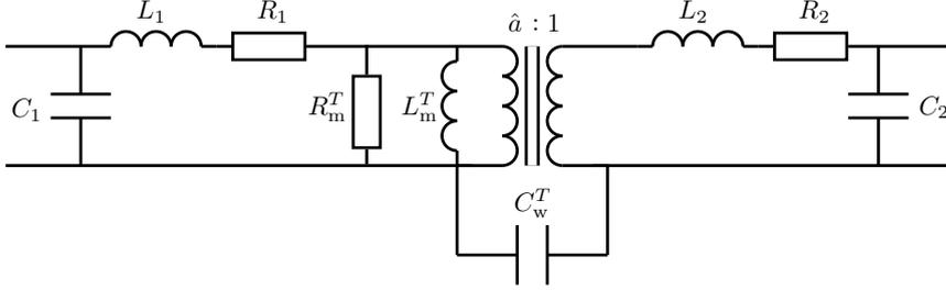
Figure 4.22: Equivalent circuit of a non-ideal transformer.
