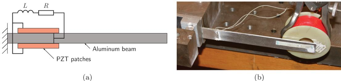
Figure 2.8: Experimental setup: (a) Cantilever beam with two collocated piezoelectric patches connected to a resonant shunt. (b) Picture of the actual setup showing the coil excitation system.
