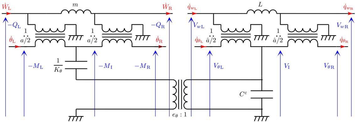
Figure 4.10: Discrete model for the electromechanical unit cell.
