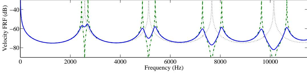
Figure 3.11: Velocity FRFs with a multimodal coupling - ( $\cdots$ ) with  $e = 0$ , ( $- \cdot -$ ) with  $e = 1$  and  $\hat{c} = 0$ , ( $—$ ) with  $e = 1$  and  $\hat{c} = 1$ .
