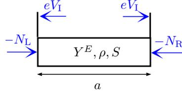
Figure 3.17: Fully homogenized model for the rod segment.
