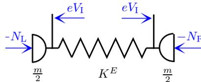
Figure 3.15: Discrete model for the rod segment.
