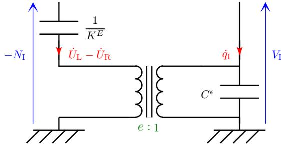
Figure 3.9: Global model of the piezoelectric unit cell.
