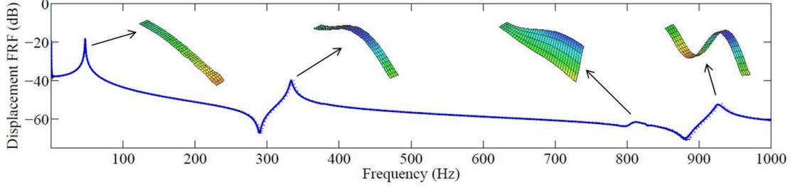
Figure 2.9: Displacement frequency response functions of the beam and corresponding operating deflection shapes obtained experimentally - (—) with short-circuited patches, ( $\cdots$ ) with open-circuited patches.
