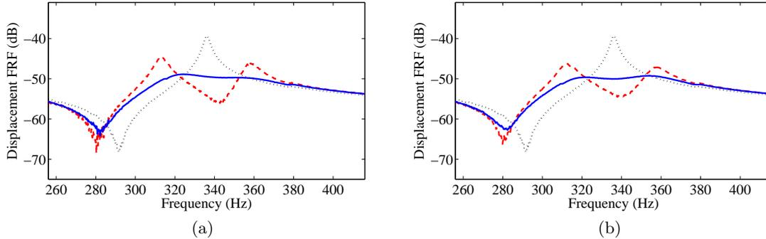
Figure 2.15: Damping of the second bending mode: (a) With the ferrite core ( $N = 613$ ) - ( $\cdots$ ) open circuit, ( $- -$ ) shunted on inductor without additional resistor, ( $—$ ) shunted on inductor with additional series resistor  $R_s^+ = 1.8 \text{ k}\Omega$ . (b) With the nanocrystalline toroid ( $N = 296$ ) - ( $\cdots$ ) open circuit, ( $- -$ ) shunted on inductor without additional resistor, ( $—$ ) shunted on inductor with additional series resistor  $R_s^+ = 1.4 \text{ k}\Omega$ .
