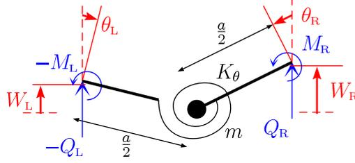
Figure 4.2: Discrete model of a beam segment.
