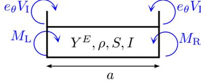
Figure 4.11: Fully homogenized model for the beam segment.
