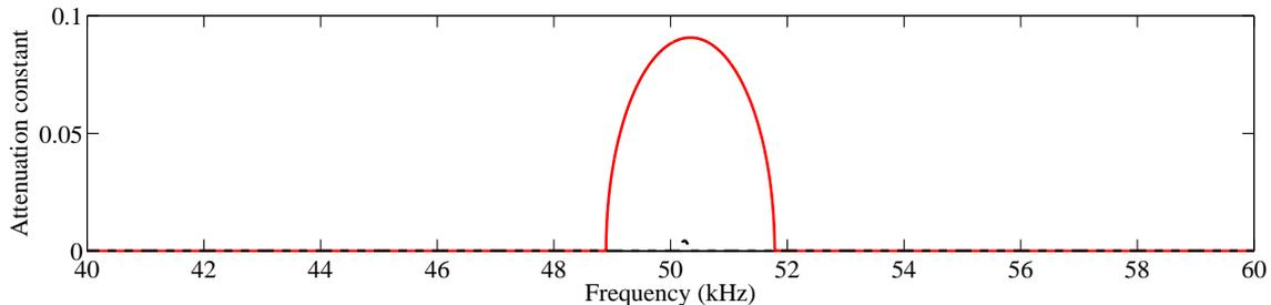
Figure 3.22: Attenuation constants - (---) for the homogenized model, (—) for the piecewise homogenized model.
