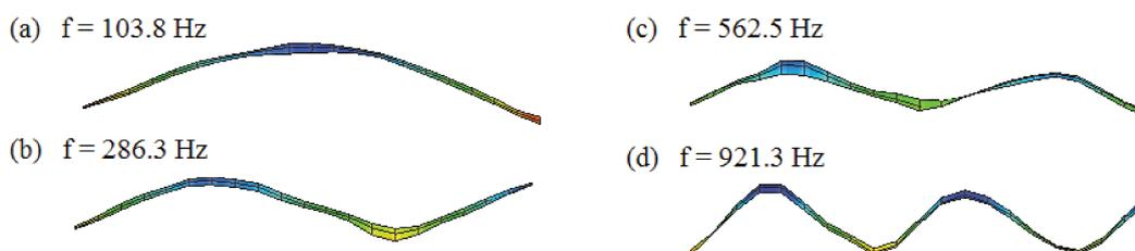
Figure 4.27: Operating deflection shapes measured with the scanning vibrometer: (a) 1<sup>st</sup> mode. (b) 2<sup>nd</sup> mode. (c) 3<sup>rd</sup> mode. (d) 4<sup>th</sup> mode.
