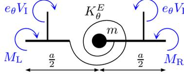
Figure 4.9: Discrete model for the beam segment.
