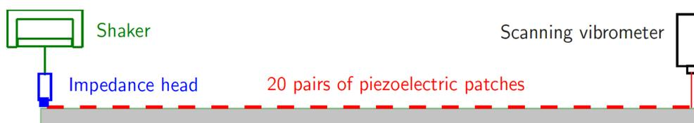
Figure 4.25: Experimental setup for the analysis of bending waves.
