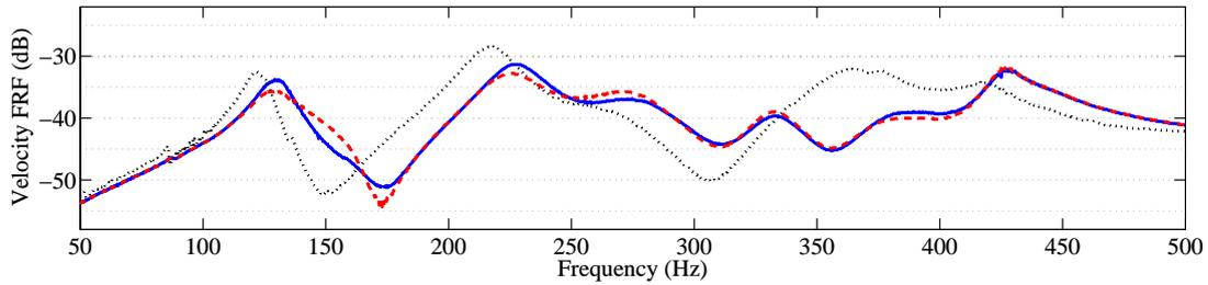
Figure 5.26: Influence of boundary conditions - (—) optimal FRF with  $L = 0.7$  H and  $R_s^+ = 180 \Omega$ , ( $\cdots$ ) with no bolts on the upper bar of the frame, (—) with the upper line of piezoelectric patches which is short-circuited.
