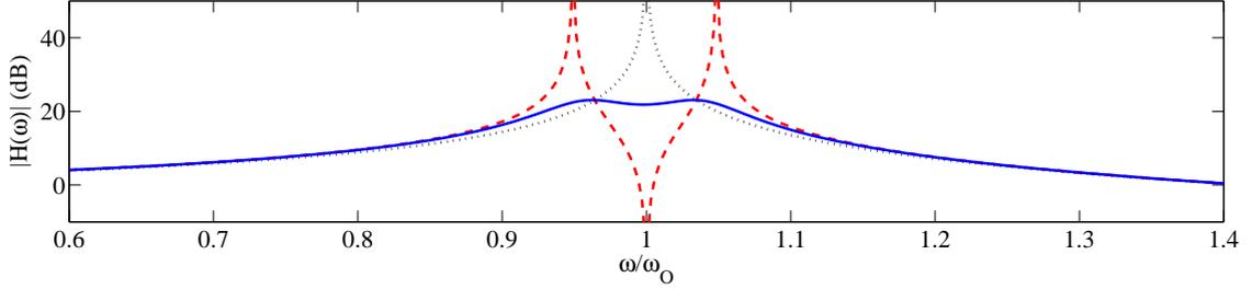
Figure 2.6: Modulus of the transfer function  $H(\omega)$  - ( $\cdots$ ) with an open circuit, ( $-\cdot-$ ) with the optimal inductance and no resistance, ( $-$ ) with the optimal inductance and the optimal resistance.
