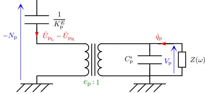
Figure 2.2: Electrical shunt of impedance  $Z(\omega)$  on a piezoelectric transducer.
