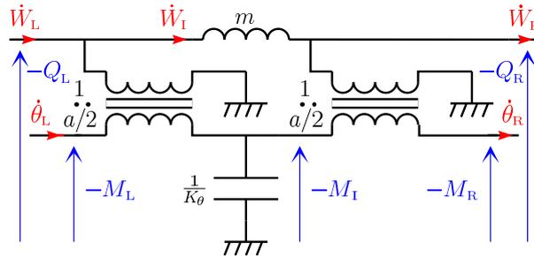
Figure 4.6: Electrical analogue of the discrete beam segment.
