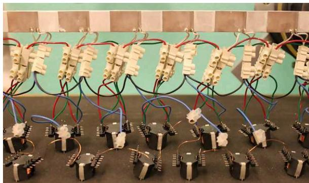
Figure 4.29: Electrical network involving inductors and transformers.
