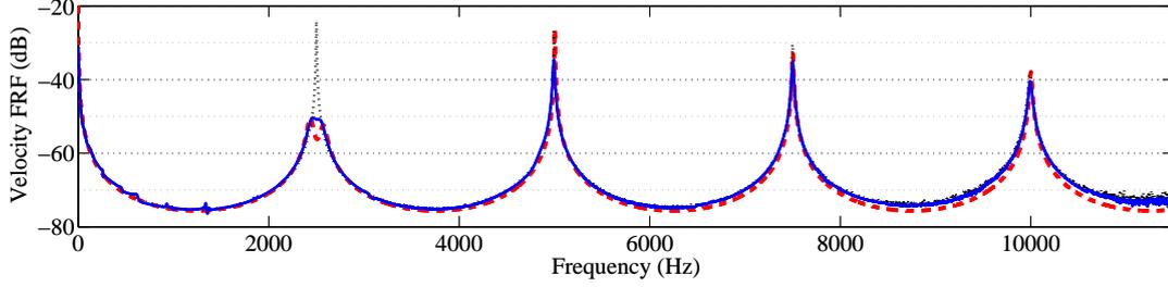
Figure 3.27: Velocity FRFs with distributed shunts - ( $\cdots$ ) for the experiment with open-circuited patches, ( $\text{—}$ ) for the experiment with resonant shunts, ( $\text{-- --}$ ) for the transfer matrix model with resonant shunts.
