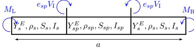
Figure 4.12: Piecewise homogenized model for the beam segment.
