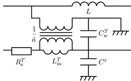
Figure 4.24: Non-ideal transformer in the analogous electrical network.
