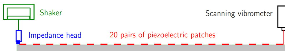
Figure 4.25: Experimental setup for the analysis of bending waves.
