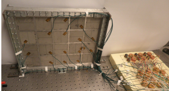
Figure 5.18: Clamped aluminum plate covered with piezoelectric patches connected to the multi-resonant network.
