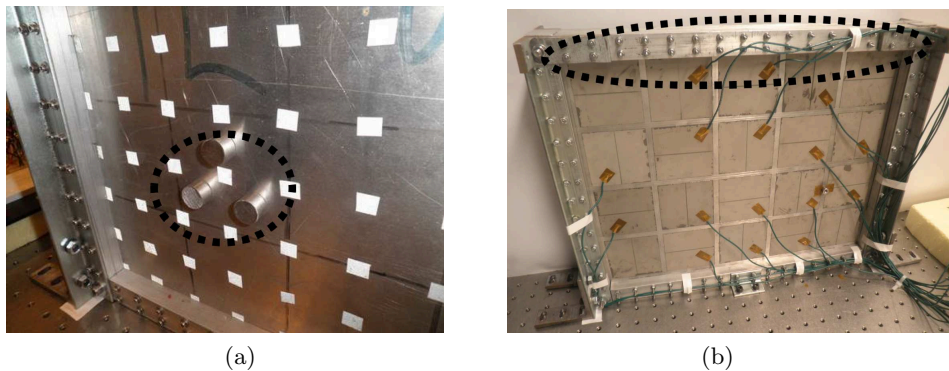
Figure 5.24: Structural modifications of the clamped plate: (a) Addition of lumped masses. (b) Loose bolts on the upper bar of the frame.
