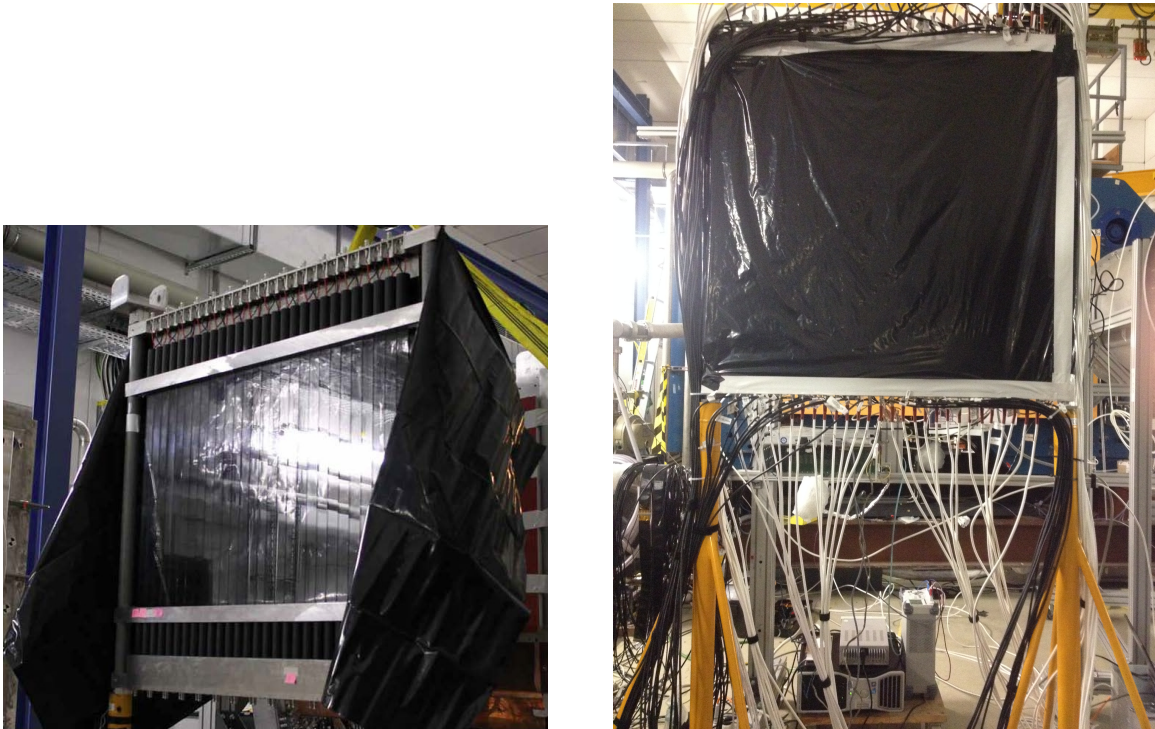
FIGURE 4.6: Pictures of the ToF wall, which is used for time of flight measurements of fission fragments. Left: vertical plastic slats and associated PMTs, with half of them placed on the top of plastics, while the rest at the bottom. Right: the operational detector is protected by the black wrapping from the interference of the light in the surrounding.
