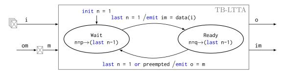
Figure 5.6: The time-based LTTA controller. A counter n is decremented in each state initialized with value p in state Wait and q in state Ready; preempted indicates that a fresh value was received on some input.
