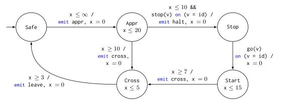
Figure 6.14: [BDL06, Figure 9] Nondeterministic train controller where x is a timer reset at each transition and id is the train identifier.
