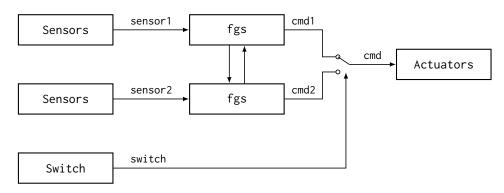
Figure 3.5: Flight guidance system. Only one FGS component, the *pilot* side is active. The crew can switch from one component to the other using a *transfer switch*.
