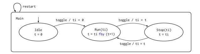
Figure 2.5: A simple stopwatch controller.
