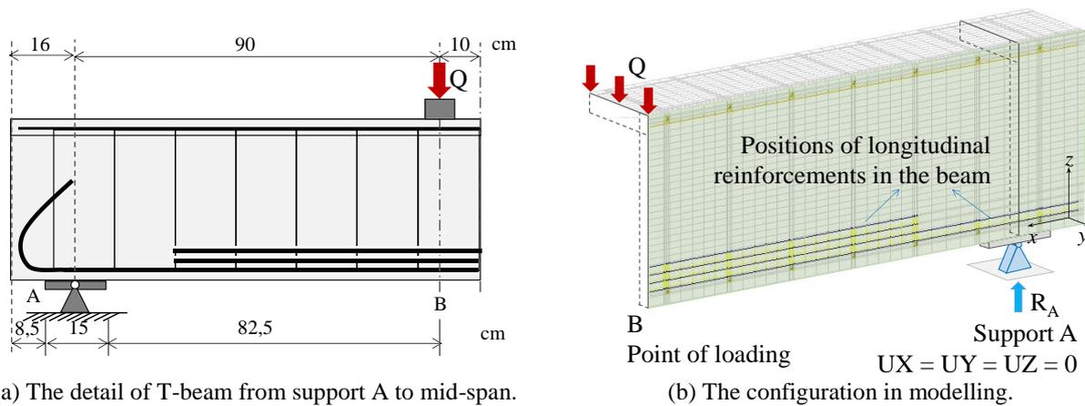
(a) The detail of T-beam from support A to mid-span.
