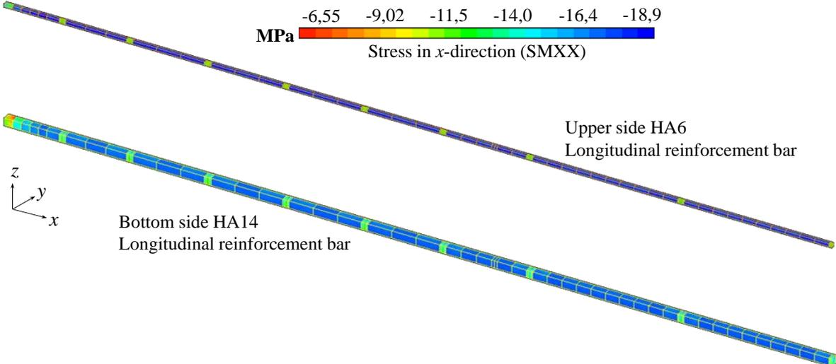
Figure 3.19. Stress field of longitudinal reinforcement at the end of shrinkage.
