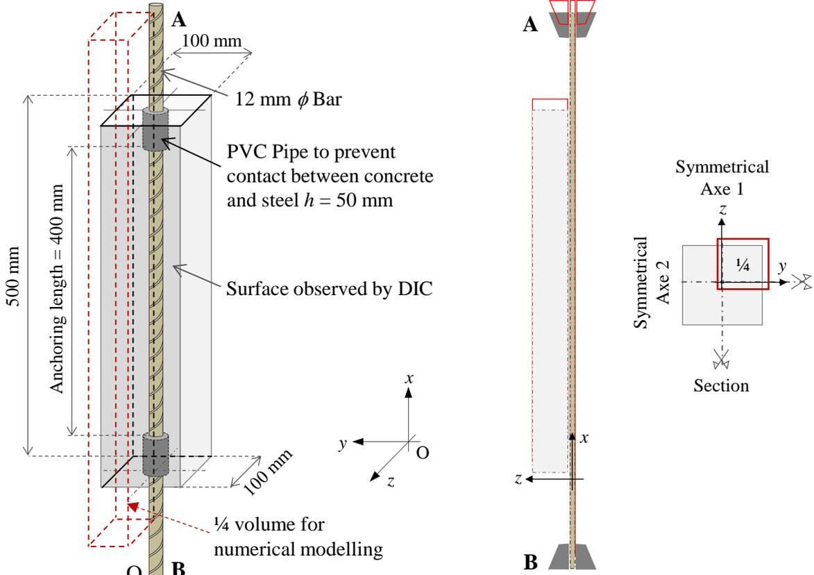
**Figure 2. 14.** Detail Dimensions of RC tensile test specimen.
