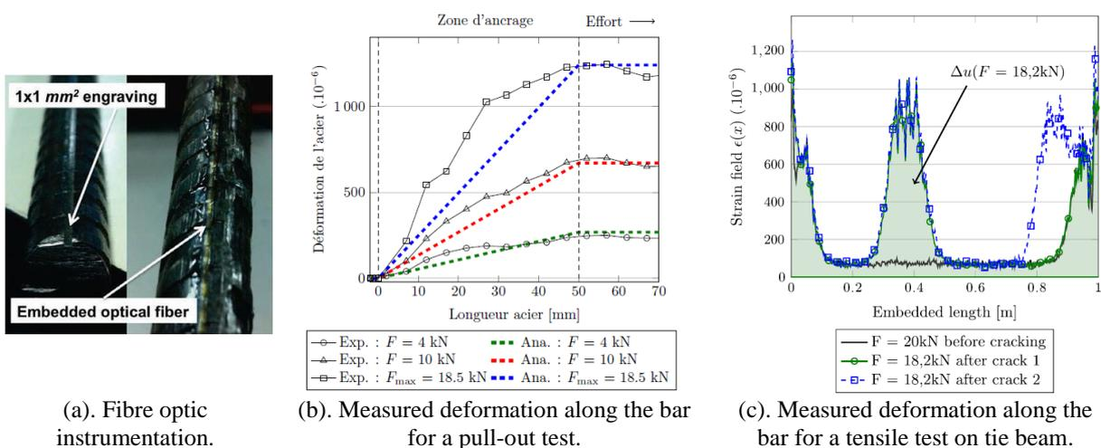
Figure 1. 8. Fibre optic instrumentation (Michou, 2015).
