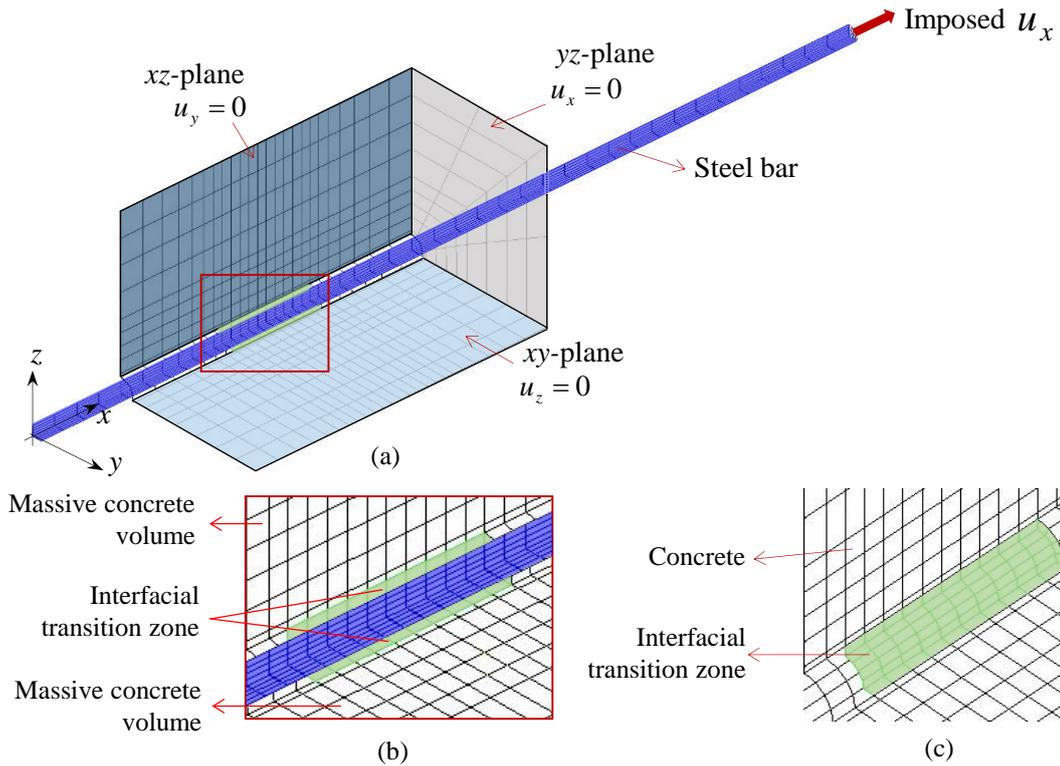
**Figure 2. 9.** Mesh and boundary conditions for pull-out test modelling (one-quarter of specimen's volume). (a) Mesh and boundary condition. (b) The detail on the anchorage length. (c) Massive concrete and interfacial transition zone along the anchorage length if steel bar does not appear.
