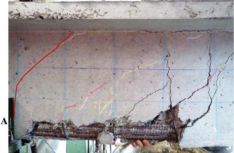
**Figure A. 15.** Cracking pattern Sample 3.
