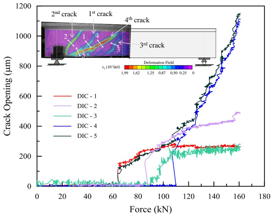
**Figure A. 8.** The evolution of crack opening observed at five different locations.
