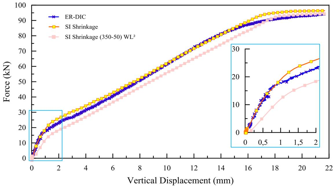
**Figure 3. 25.** Global behaviour: Experimental (ER-DIC), Modelling SI (Sliding Interface) + Shrinkage ( $350\mu\text{m/m}$ - $50\mu\text{m/m}$ ); and SI + Shrinkage ( $350\mu\text{m/m}$ - $50\mu\text{m/m}$ ) +  $WL^2$  results.
