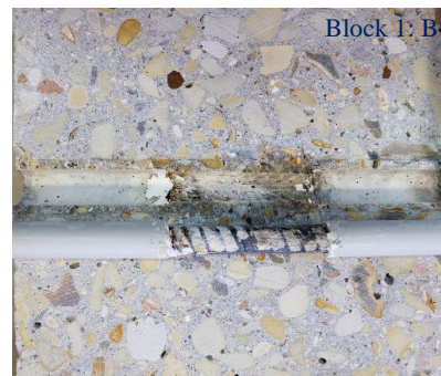
(c) Block 1 with detached steel bar
