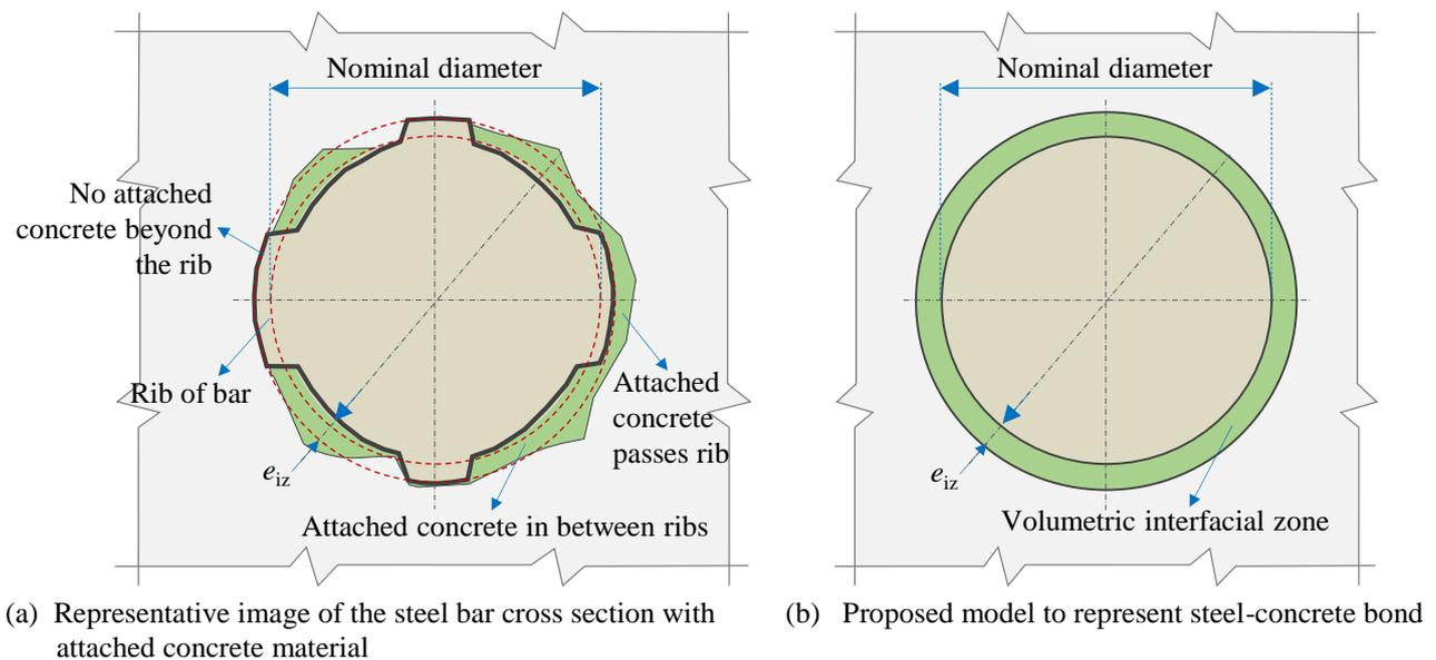
**Figure 2.7.** Sketch of the attached concrete around steel bar and the proposed geometry for numerical simulation.
