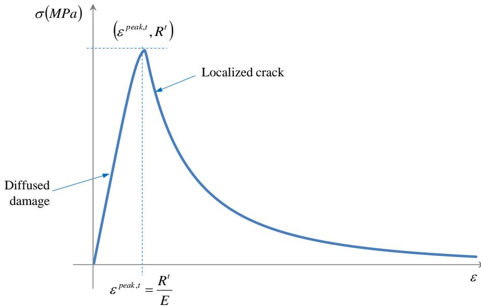
**Figure 1. 16.** Behaviour law under tension loading: test on one CUB8 element.
