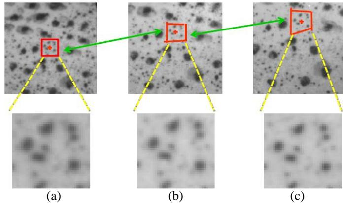
**Figure 1.6.** Images following the speckle pattern on the specimen.
