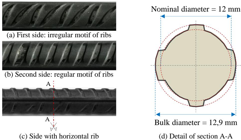
**Figure 2. 1.** Detail of steel bar reinforcement.**Table 2. 3.** Mechanical properties of steel reinforcement bar.
