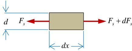
Figure 2. 26. Force in one element of reinforcement.
