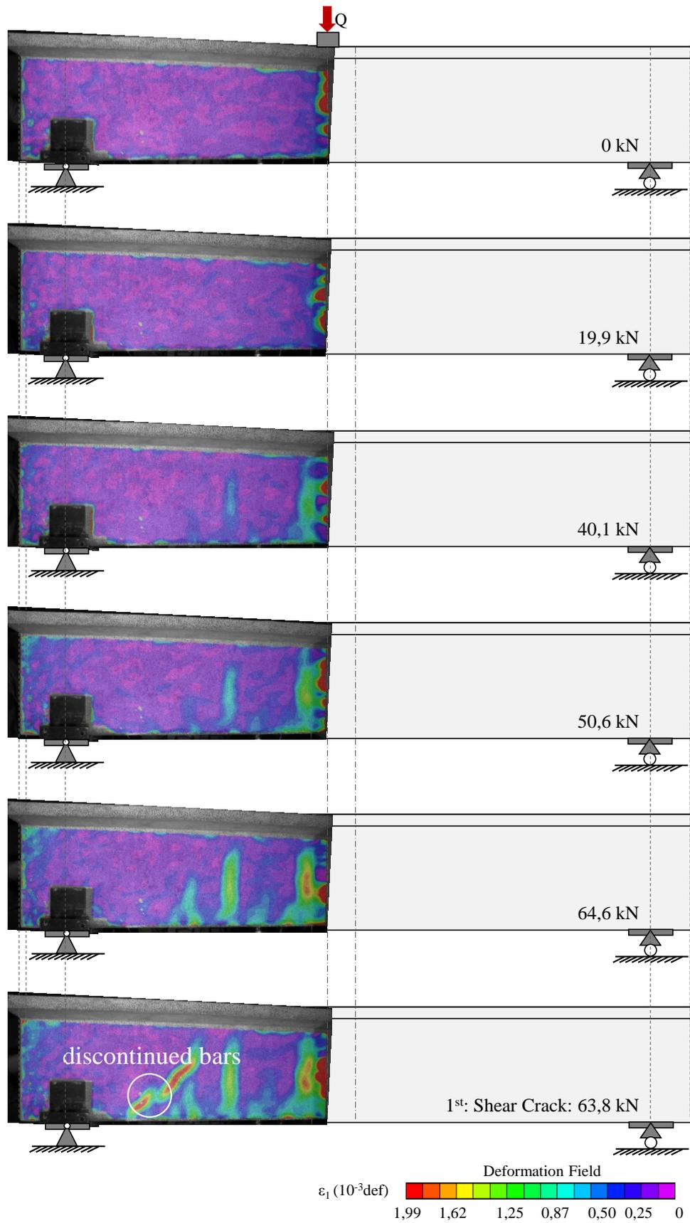
(a). Evolution from 0 to 63,8 kN (1<sup>st</sup> Shear Crack).
