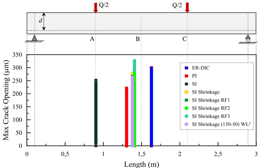
Figure 3. 31. The position of the maximum crack opening for each case of calculation at 50,5 kN.
