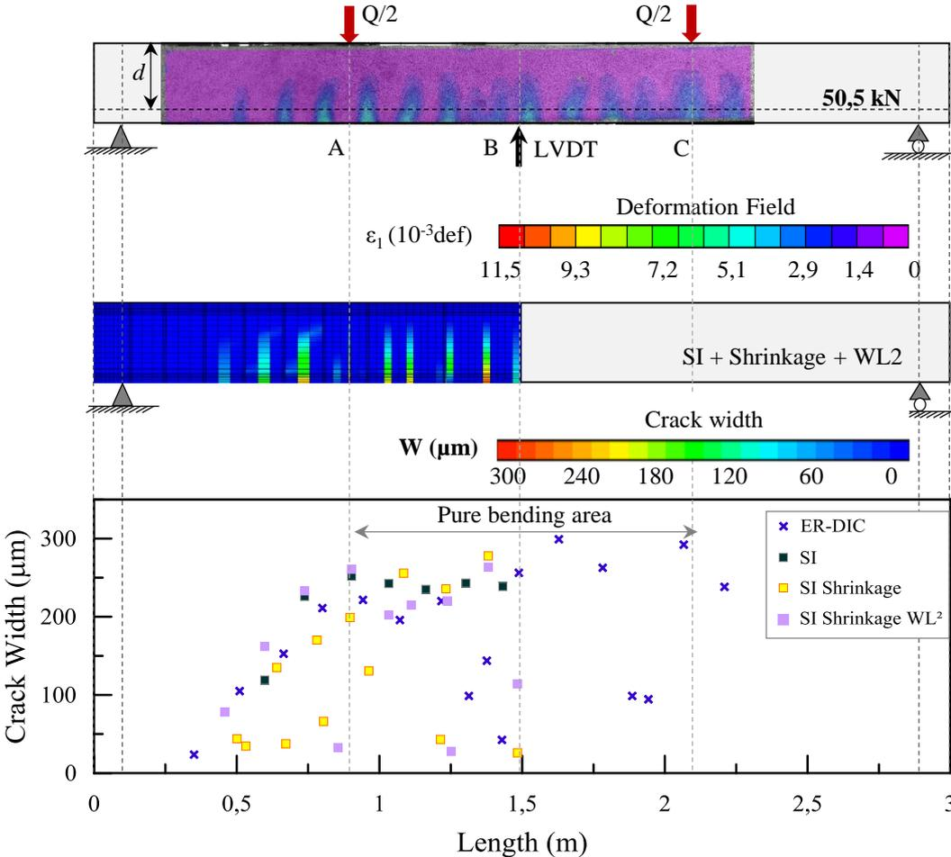
**Figure 3. 27.** Cracking pattern and opening at 50,5 kN: Experimental (ER-DIC), Modelling SI (Sliding Interface) + Shrinkage (350μm/m-50μm/m); and SI + Shrinkage (150μm/m-50μm/m) + WL<sup>2</sup> results.
