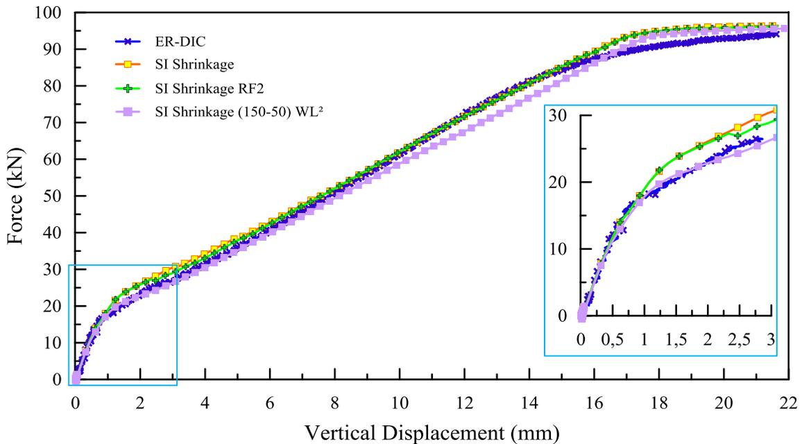
**Figure 3. 28.** Global behaviour: Experimental (ER-DIC), Modelling SI (Sliding Interface) + Shrinkage (350 $\mu$ m/m-50 $\mu$ m/m); SI (Sliding Interface) + Shrinkage (350 $\mu$ m/m-50 $\mu$ m/m) + TBM; and SI + Shrinkage (150 $\mu$ m/m-50 $\mu$ m/m) +  $WL^2$  results.
