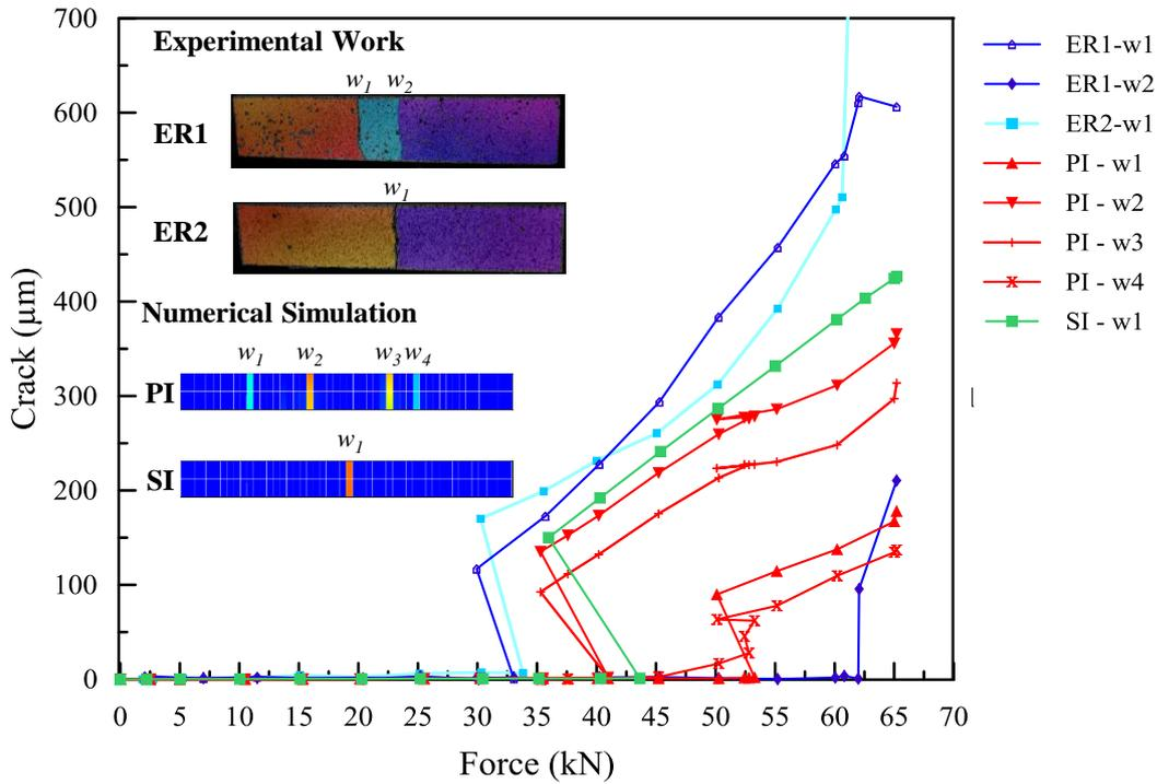
Figure 2. 23. Evolution of crack width for each crack.
