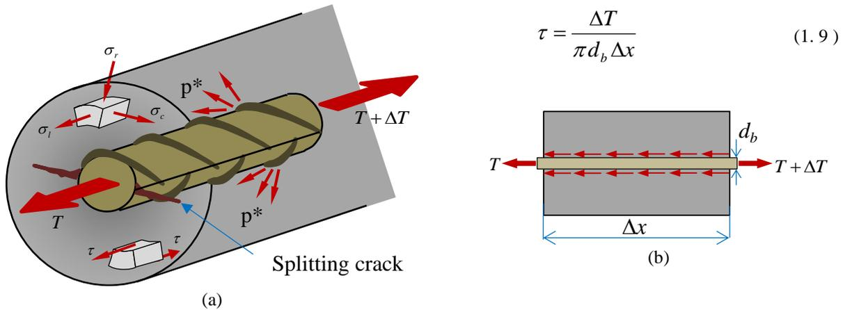
**Figure 1. 11.** Bond stress in the interfacial zone.
