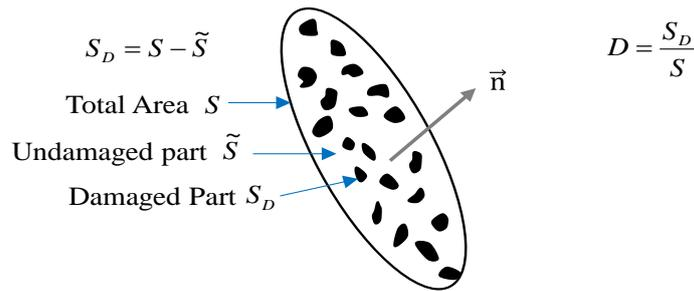
**Figure 1.14.** A representative area of a damaged solid.
