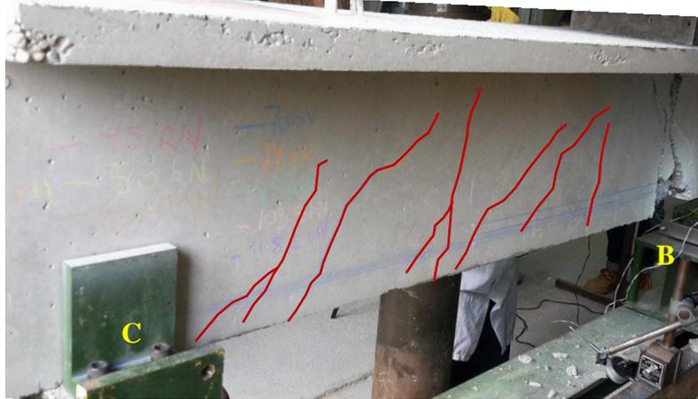
**Figure A. 16.** Cracking pattern Sample 4.
