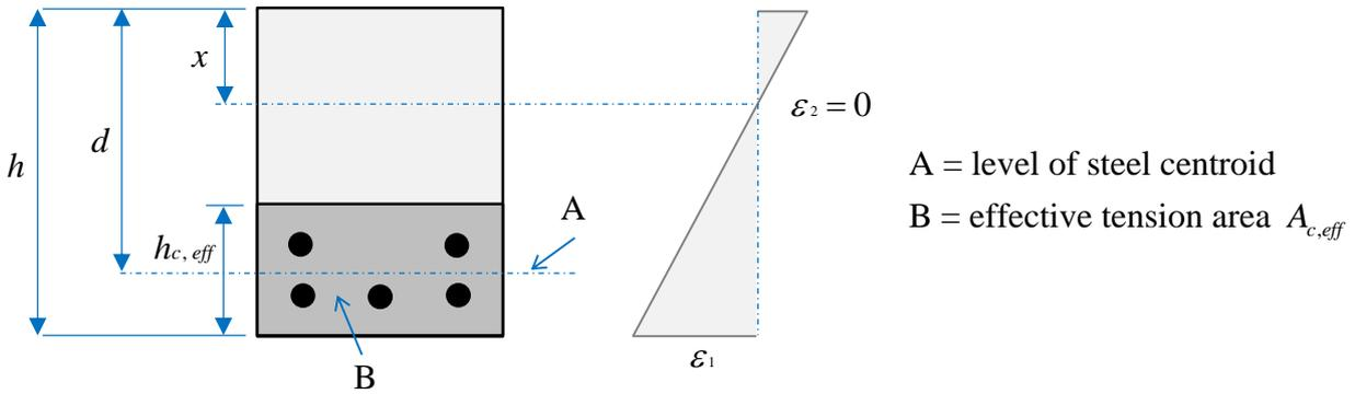
Figure 1. 1. Effective tension area for a beam case (Eurocode 2, 2005).
