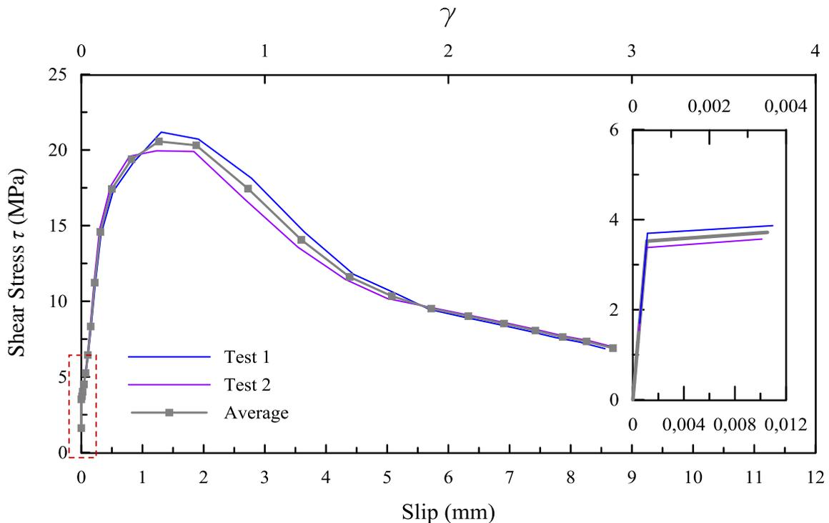
**Figure 2. 4.** Pull-out test: experimental results.
