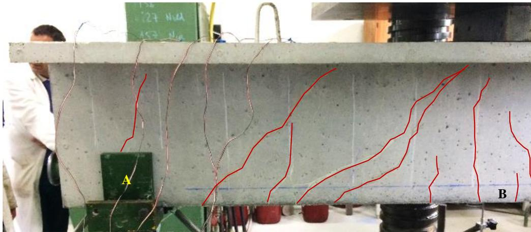
**Figure A. 17.** Cracking pattern Sample 5: A to B.
