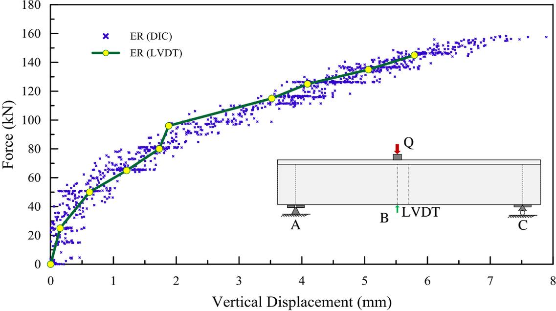
Figure A. 5. Global behaviour, vertical displacement  $U_z$  under the loading application of T-beam measured by LVDT extensometer and DIC.
