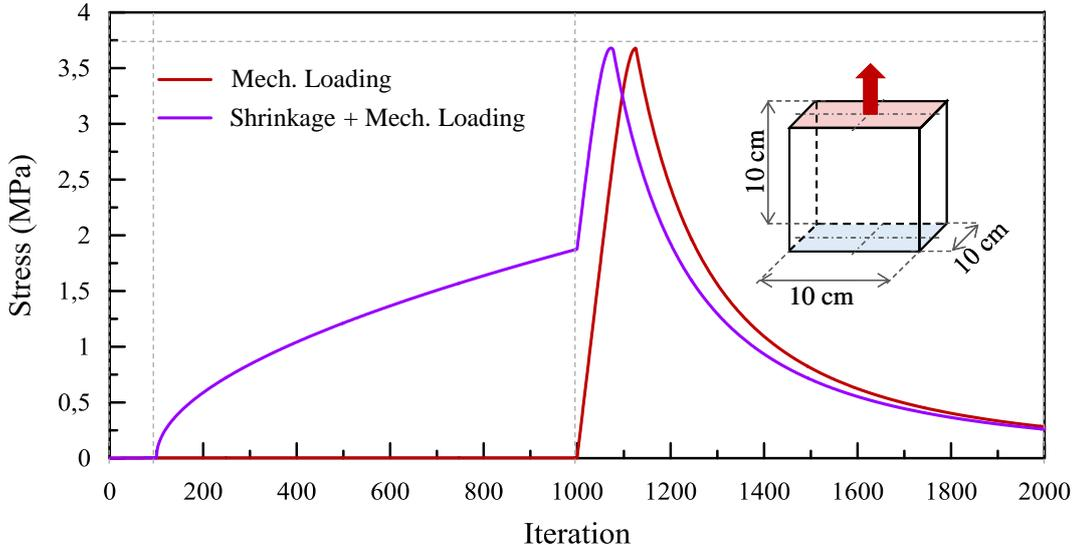
**Figure 3. 17.** The response of material under shrinkage and mechanical loading in force-iteration number curve: comparison of the pre-dried cube (purple) to the moist cube (brown).
