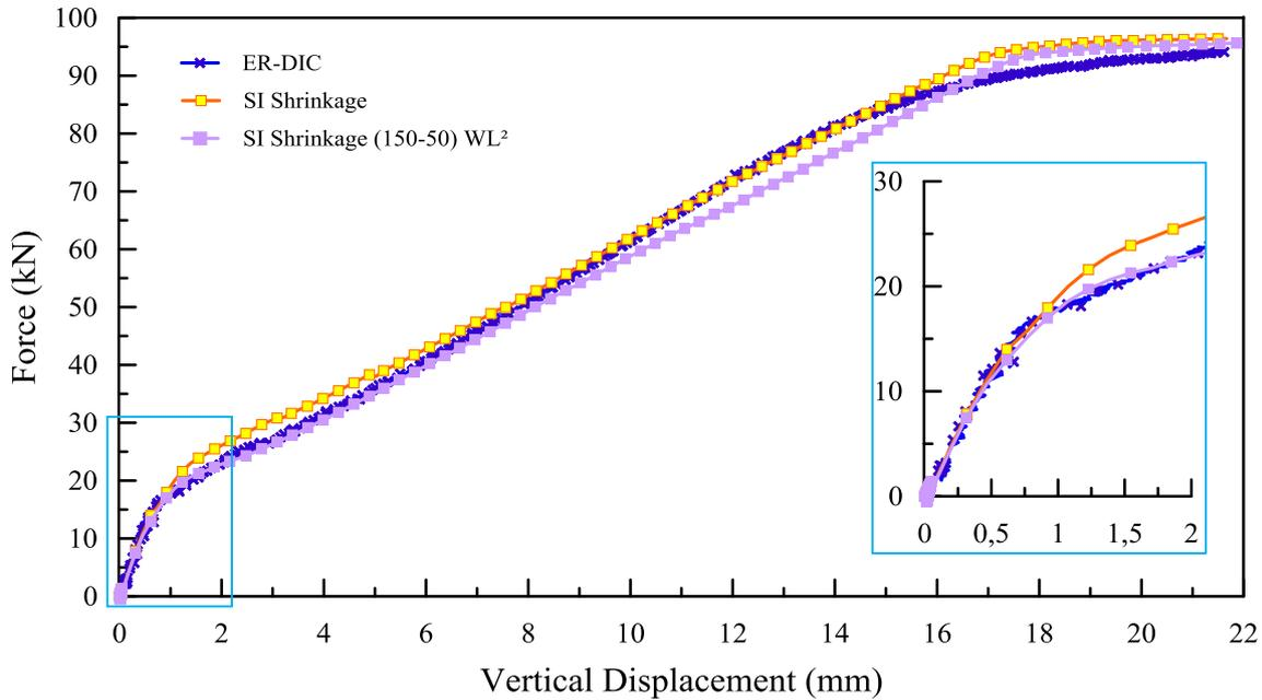
**Figure 3. 26.** Global behaviour: Experimental (ER-DIC), Modelling SI (Sliding Interface) + Shrinkage (350 $\mu\text{m}/\text{m}$ -50 $\mu\text{m}/\text{m}$ ); and SI + Shrinkage (150 $\mu\text{m}/\text{m}$ -50 $\mu\text{m}/\text{m}$ ) + WL<sup>2</sup> results.
