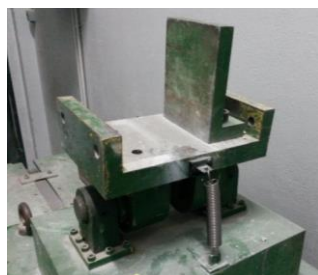
(c) Support A: Pin support.
