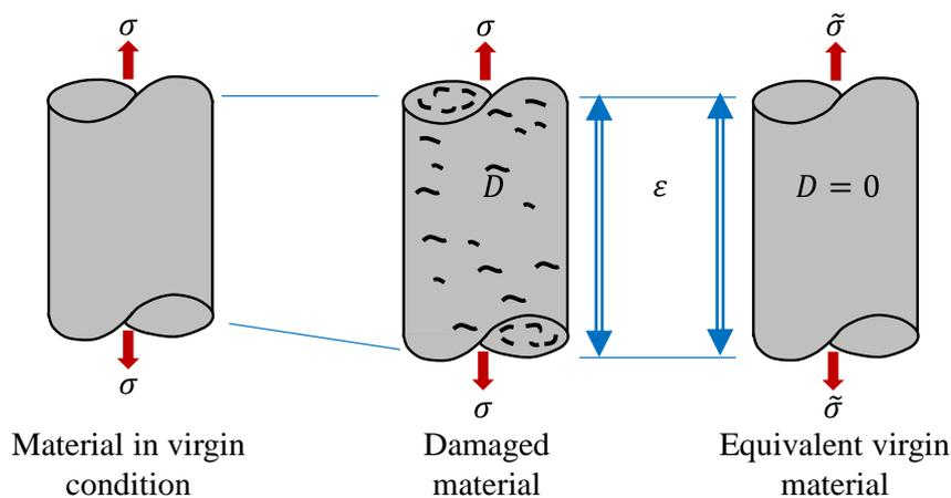
**Figure 1.15.** Effective stress and strain-equivalence principle.
