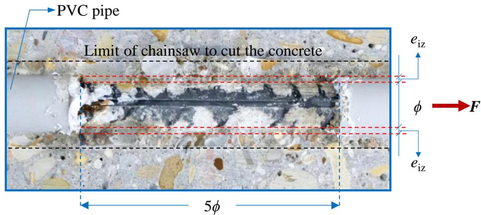
$e_{iz}$  = thickness of deteriorated concrete layer
