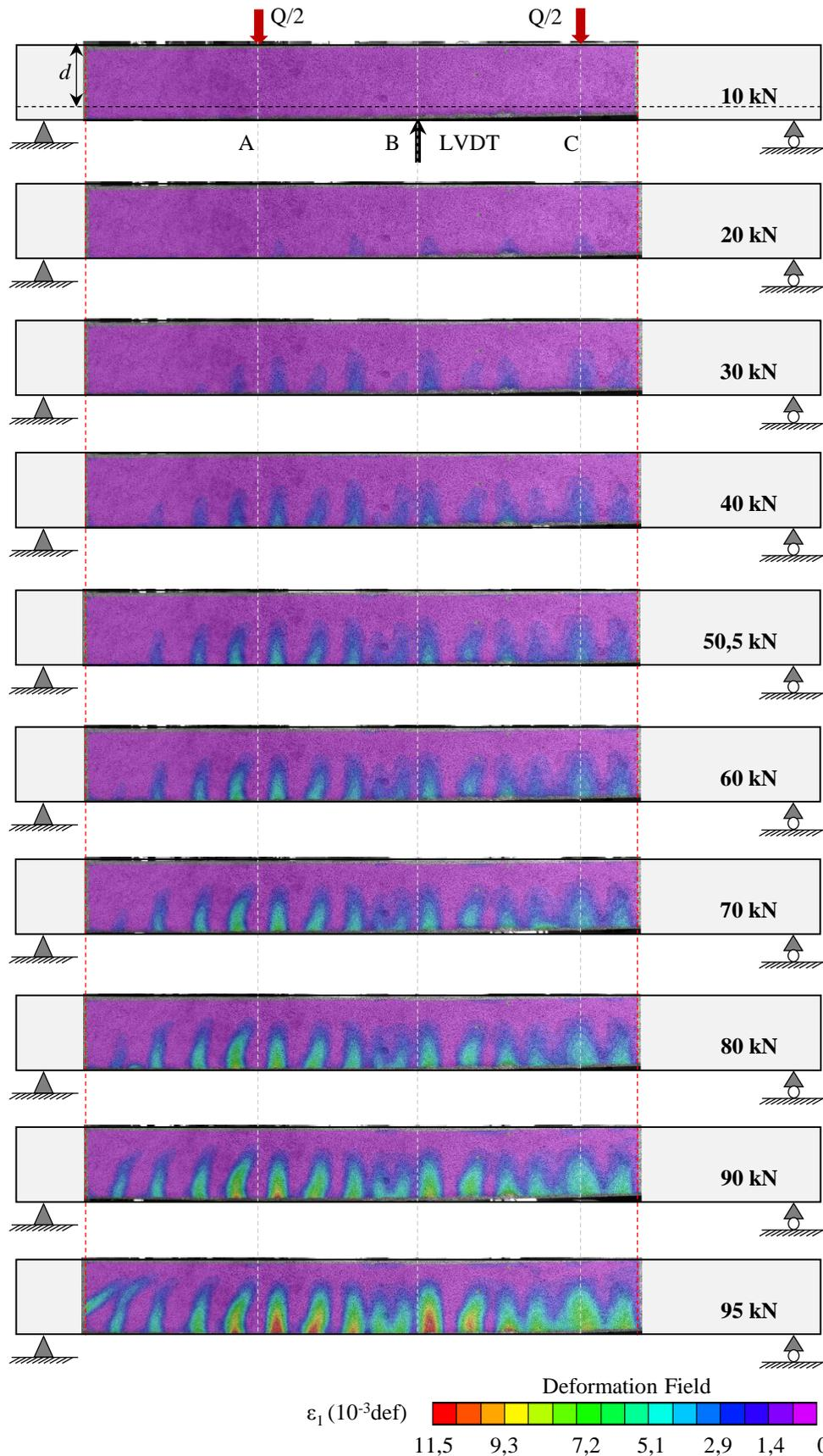
**Figure 3. 7.** Experimental results (DIC): evolution of cracking pattern observed on deformation field in major direction ( $\varepsilon_1$ ).
