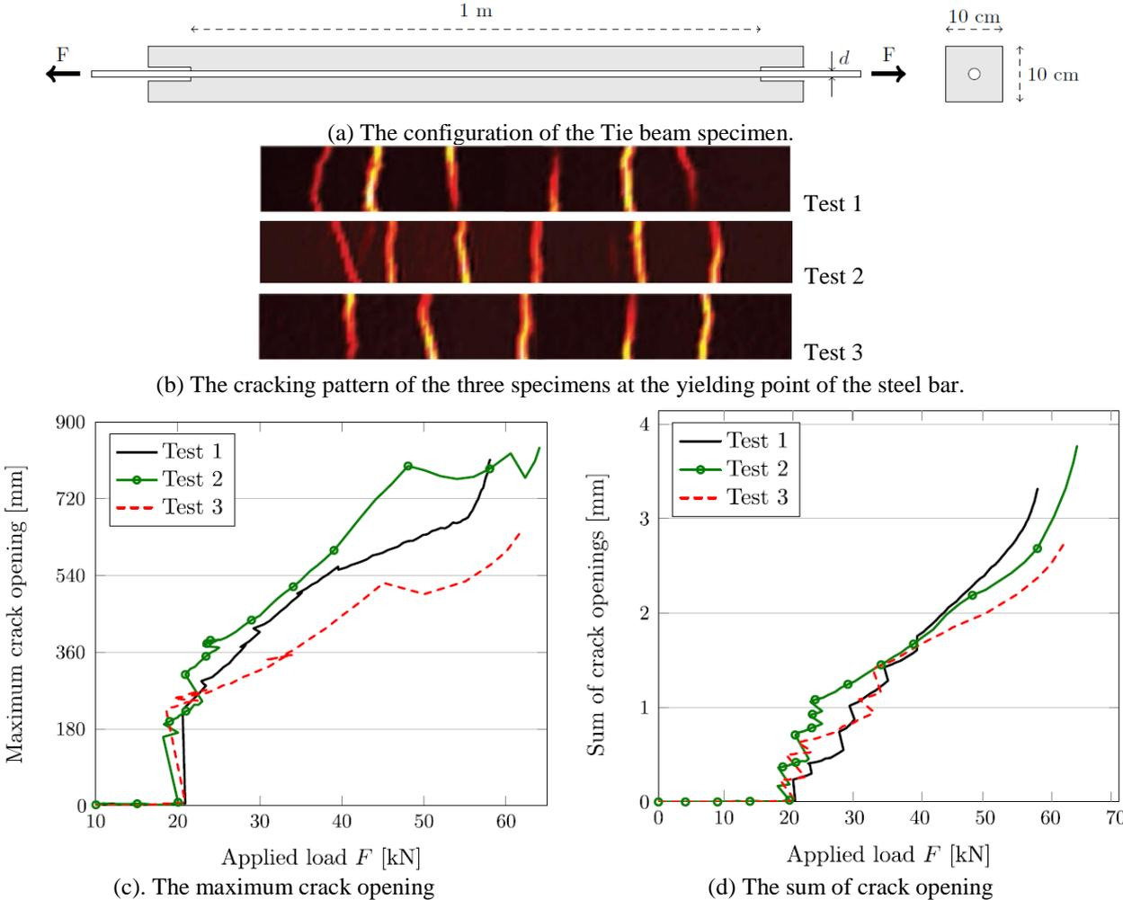
Figure 1. 3. Tensile test results from (Michou et al., 2015).
