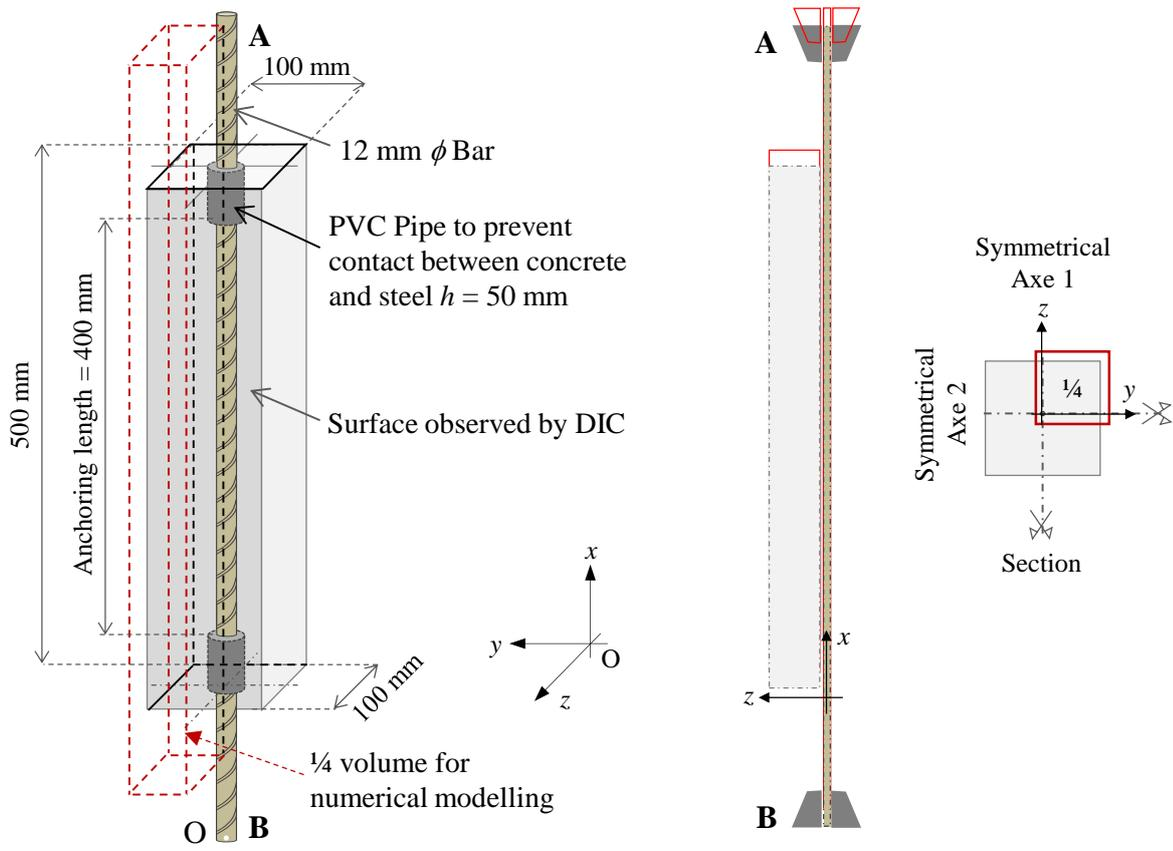
Figure C. 1. Detail of dimension for tensile test.
