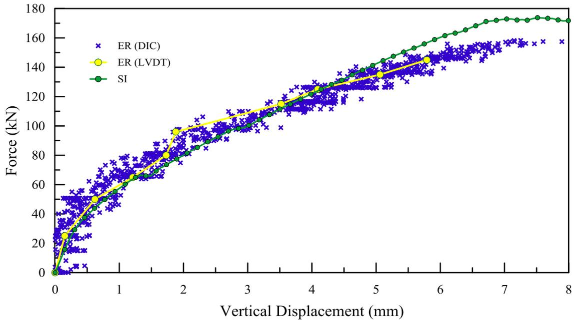
**Figure A. 12.** Global behaviour: Experimental (ER-DIC and ER-LVDT), Modelling SI (Sliding Interface) results.
