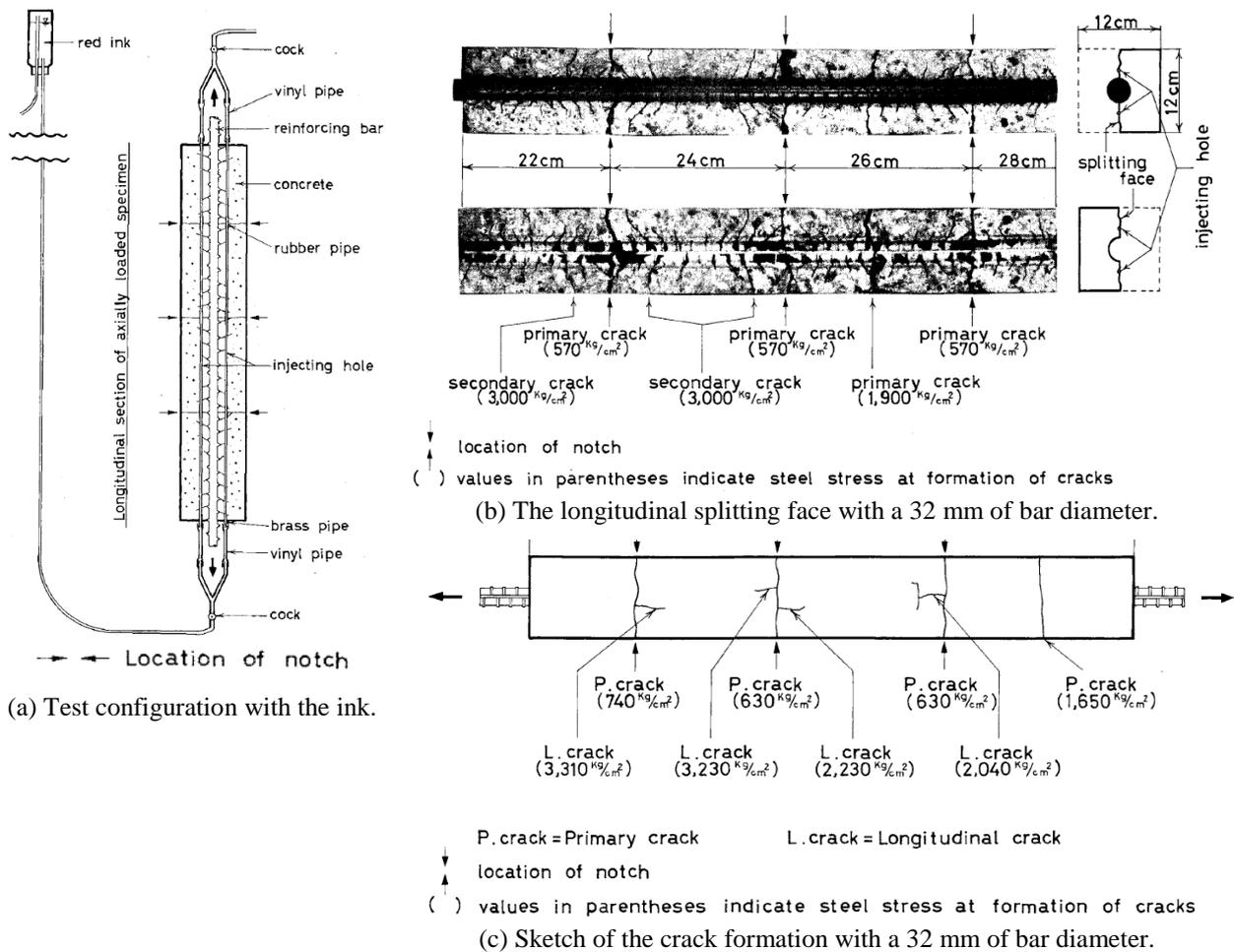
Figure 1. 2. Tensile test of Goto. (Goto, 1971).
