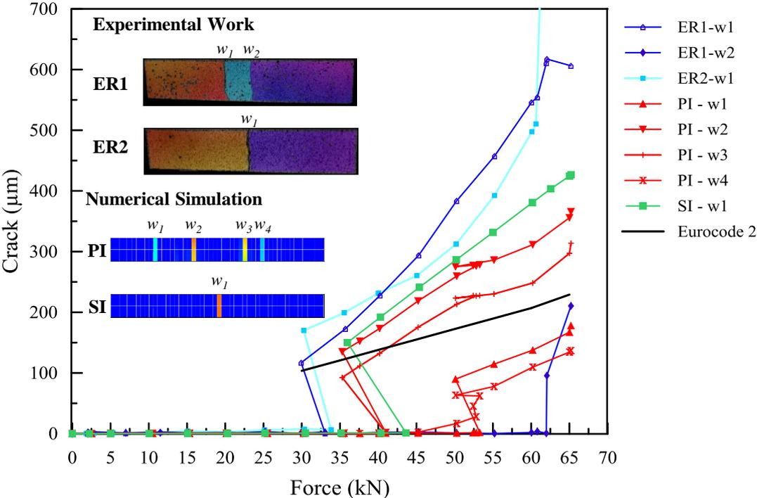
Figure C. 2. Evolution of the maximum crack width with  $S_{r,max} = 13 \text{ cm}$ .
