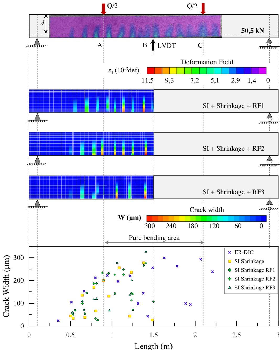
**Figure 3. 24.** Cracking pattern and opening at 50,5 kN: Experimental (ER-DIC), Modelling SI (Sliding Interface) + Shrinkage; and SI + Shrinkage + TBM results.
