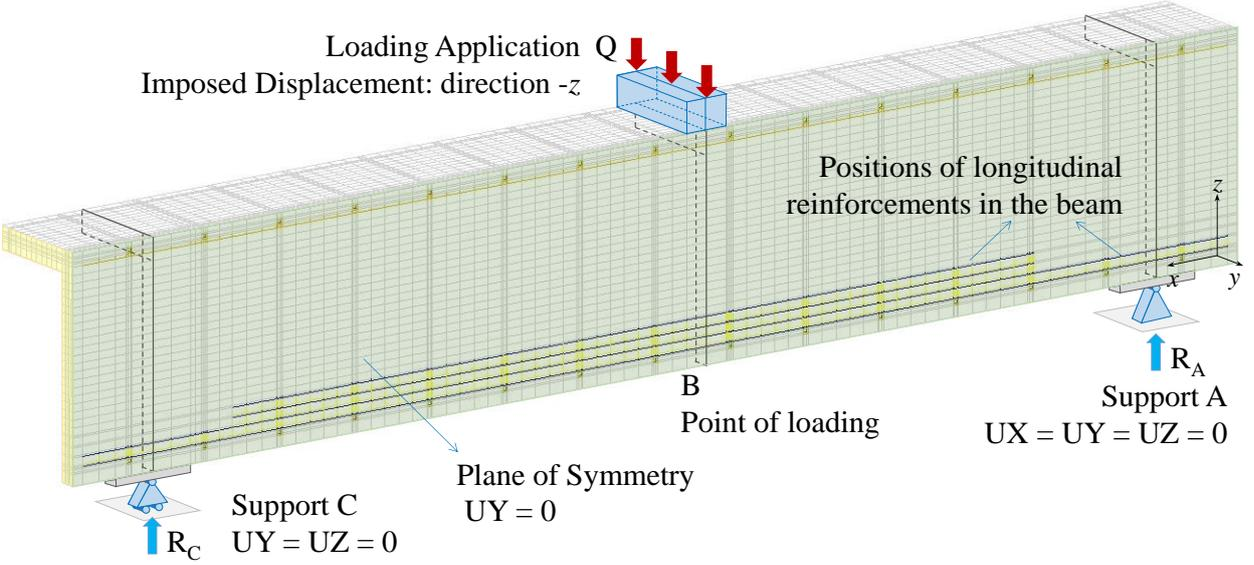
(b). Detail of a half RC T-beam volume: 2<sup>nd</sup> point of view.
