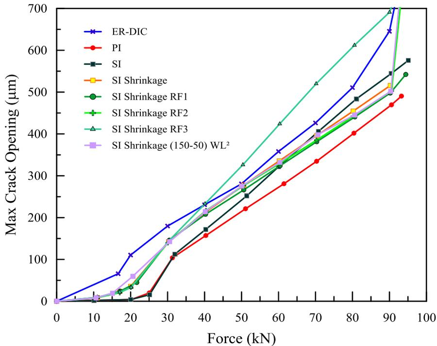
**Figure 3. 29.** The evolution of  $w_{\max}$  during loading, experimental and simulations comparison.
