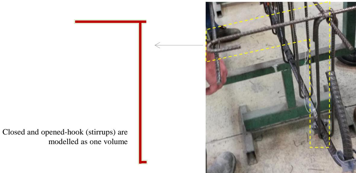
**Figure A. 10.** Mesh and boundary conditions for modelling: a half of specimen's T-shaped section.
