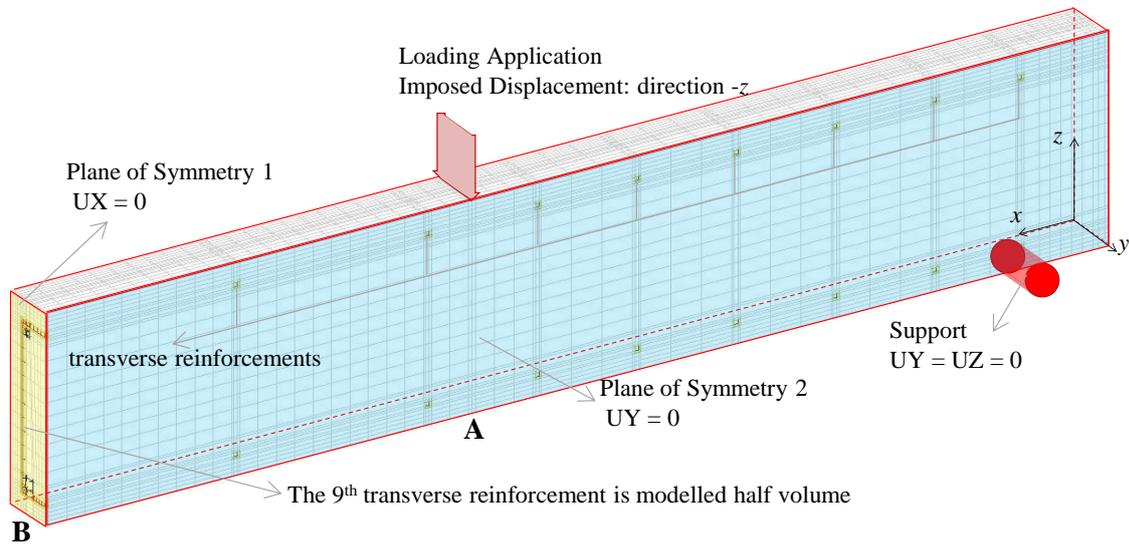
(a) Detail of one-quarter volume of RC beam. A-B indicates the pure bending area.
