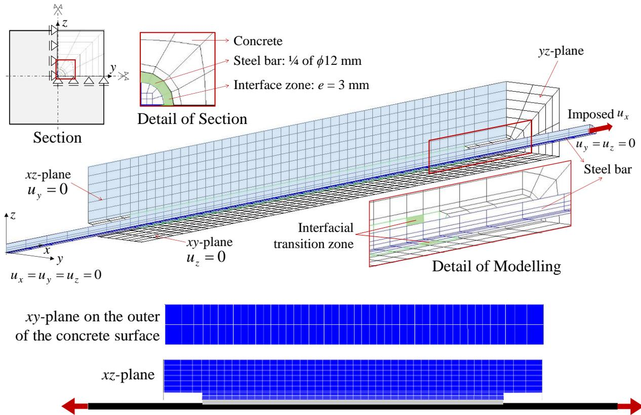
Figure 2.16. Mesh and boundary conditions for modelling (one-quarter of specimen's volume).
