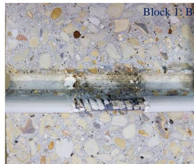
(c) Block 1 with detached steel bar
