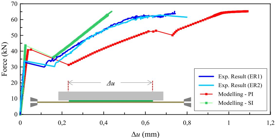
Figure 2. 19. Force-delta displacement in global behaviour.
