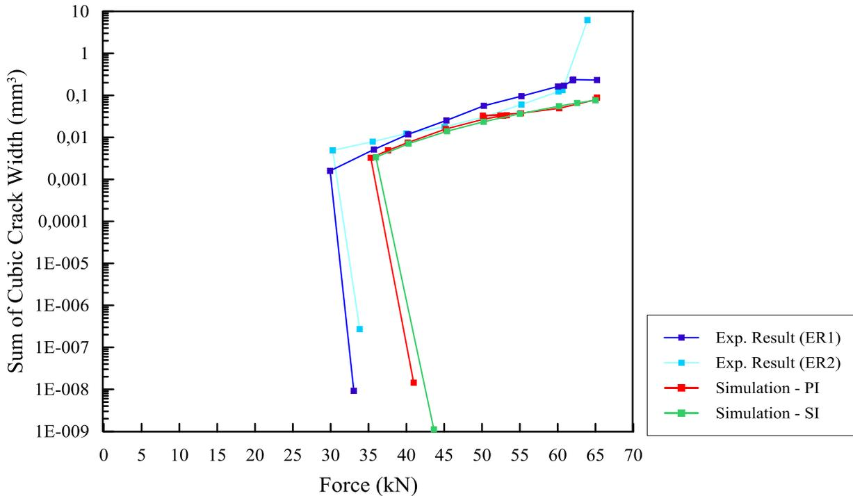
Figure 2. 24. Evolution of crack width for each crack.
