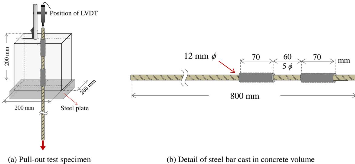
Figure 2. 2. Detail of specimen in the Pull-Out test.
