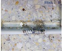
(c) Block 1 with detached steel bar
