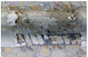
(d) Block 2 without attached bar (e) Zoomed part of picture (c) Block 1 **Figure 2. 5.** Cutting through concrete on the pull-out test specimen.
