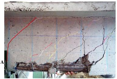
Figure A. 15. Cracking pattern Sample 3.
