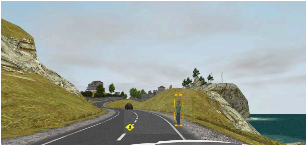
Figure 4.4.7: Display of the bounding box and the warning panel when the driver is unaware of the pedestrian at the critical moment.
