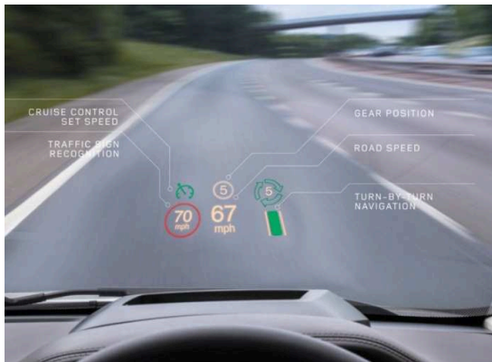
Figure 4.1.3: Integrated windshield HUD concepts [Rover 15][Continental 15].
