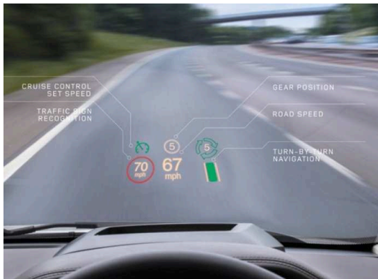
Figure 4.1.3: Integrated windshield HUD concepts [Rover 15][Continental 15].
