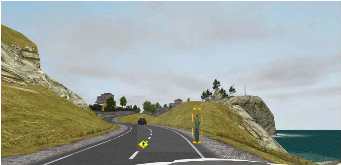
Figure A.4: HUD Pedestrian is augmented by a bounding box, and the warning panel is displayed in the critical moment
