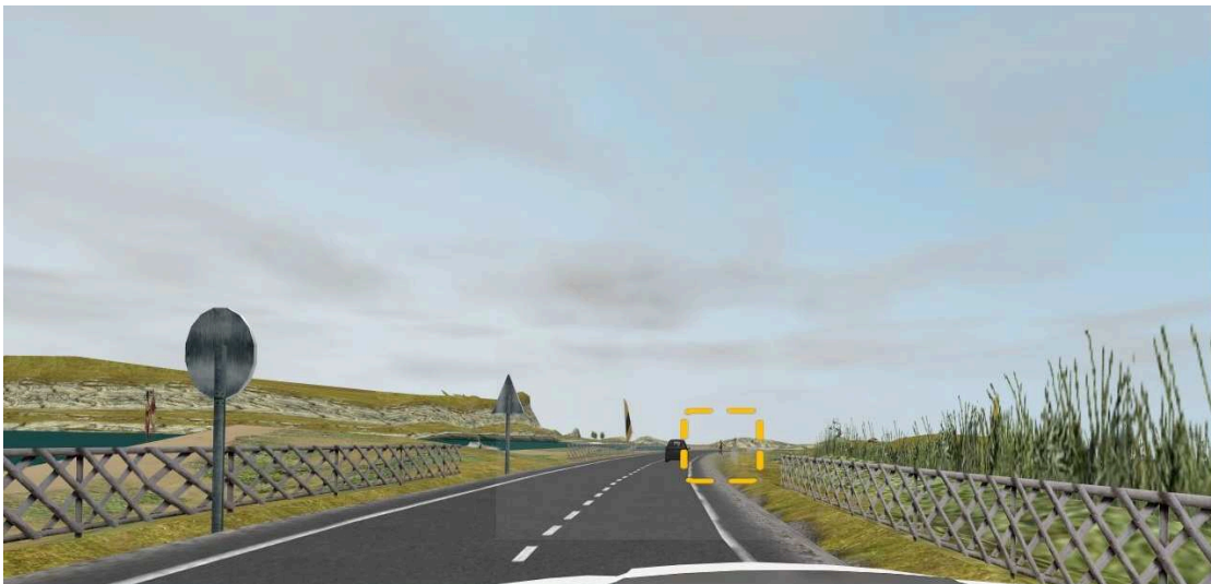
Figure A.3: Pedestrian is augmented by a bounding box
