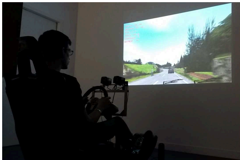
(b) The visual module with a projector screen.
