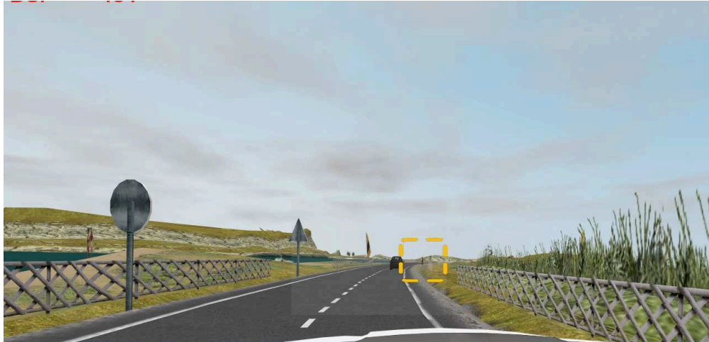
Figure 4.4.6: Display of the bounding box when the pedestrian is detected far from the car.
