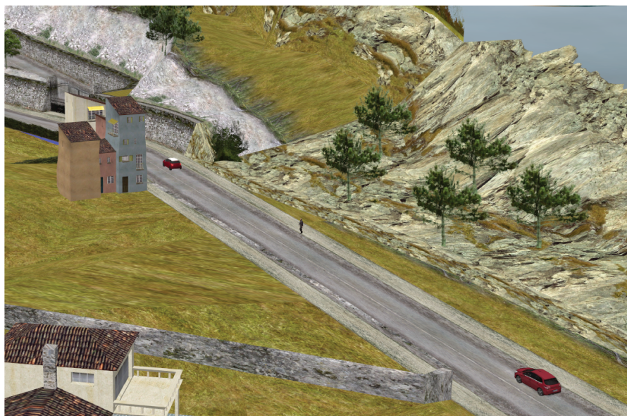
Figure 5.1.4: 3D View of the Scenario (Step 3): When the distance between the test vehicle and the pedestrian is 30m. The pedestrian can be randomly activated to cross the road.
