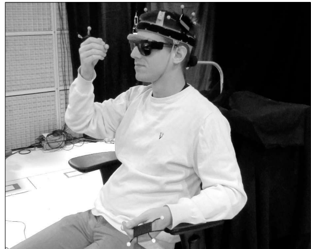
Figure 1. Photo of the proximal pointing task. The participant holds a rigid body in each hand, aligning the reference marker with his fingertips. The head is supported by a neck-rest to prevent head movements, and the head position and orientation were monitored in real-time using the motion capture system (inner frame of a helmet with reflective markers). The subjects were free to use the hand of their choice according to the most comfortable way to indicate the direction of the sound source, which is computed with regard to the current head position.
