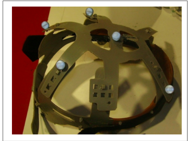
Figure 2: Safety helmet frame with reflective markers for head motion capture.
