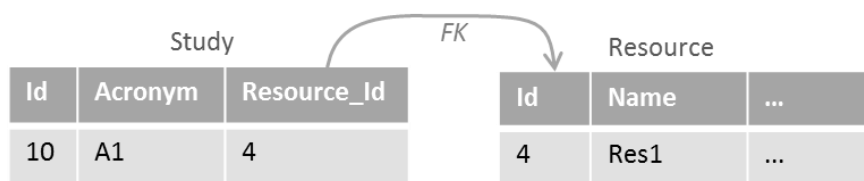
Figure 7: Relational schema with a cross-reference
