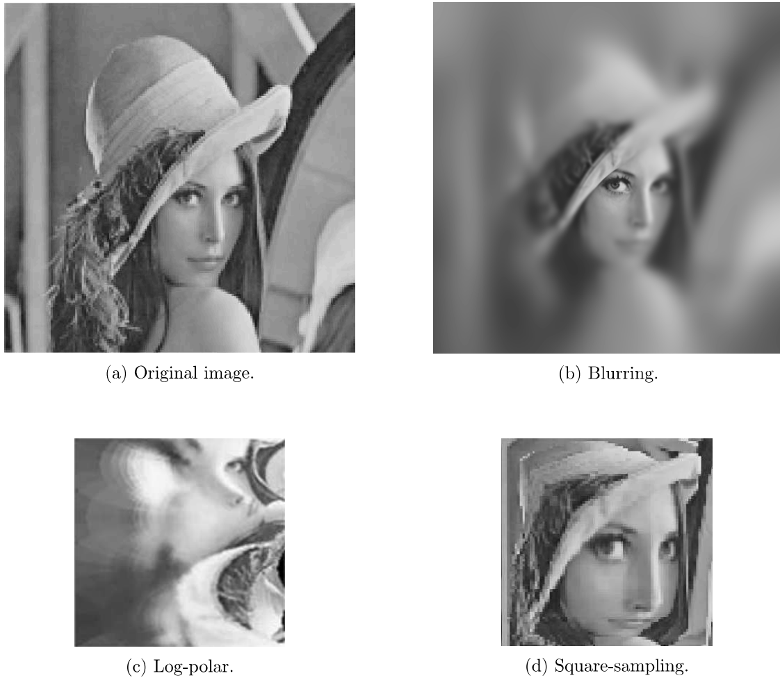
Figure 2-1: Some of the classical methods traditionally used for emulating retinal sampling and cortical images. Notice that blurring in (b) keeps the same number of pixel as in the original image. The log-polar and the square-sampling methods in (c) and (d) introduce severe spatial deformations that make further spatial filtering more challenging.
