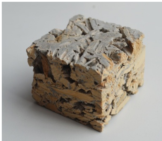
Figure IV. 8: Matériau d'étude: composite bois-ciment
