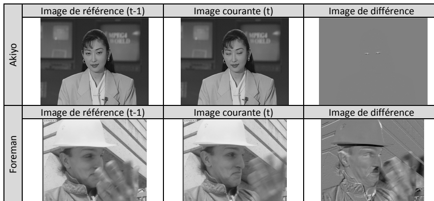
Figure 1.3. Illustration du principe de codage FD (Frame Difference)
