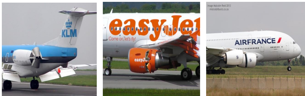
a) Bucket type (Source: Fokker70, KLM) b) Clamshell door type (Source: Airbus A320, Easyjet) c) Translating cowl type (Source: Airbus A380, AirFrance)
