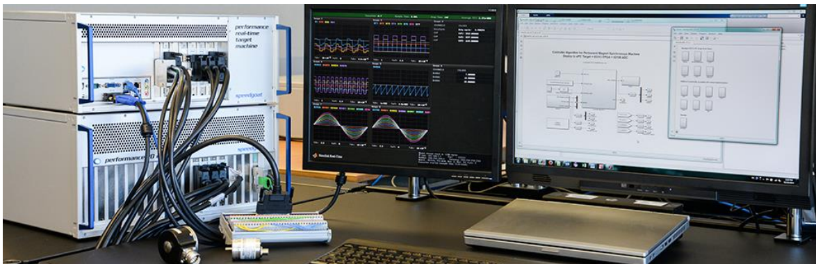
Fig. 5-7 Speedgoat program environment (MATLab/Simulink) and real-time display [3]
