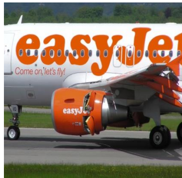
b) Clamshell door type (Source: Airbus A320, Easyjet)
