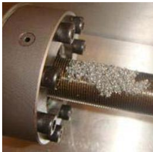
Fig. 4-10 Airbus Jamroll project for study jamming issue on roller screw [13]
