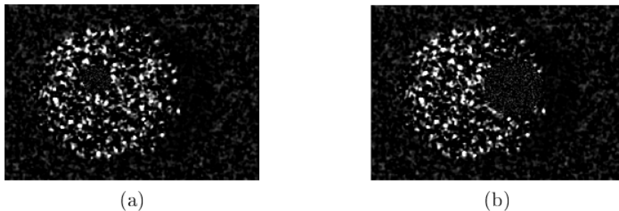
Figure A.1: Example of PolSARproSim outlier images containing (a) 5% and (b) 20% of aberrant pixels.
