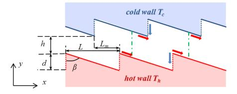
Figure 5.12: Configuration and geometric parameters
