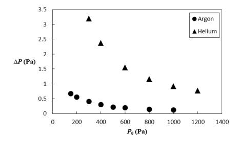
Figure 4.14: Pressure difference versus operating pressure for a 2-stage pump  $(T_c=77~{\rm K},T_h=370~{\rm K}~).$
