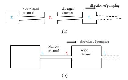
Figure 3.10: Configuration of a Knudsen pump with tapered channels (a) compared to the configuration of classic Knudsen pump (b)
