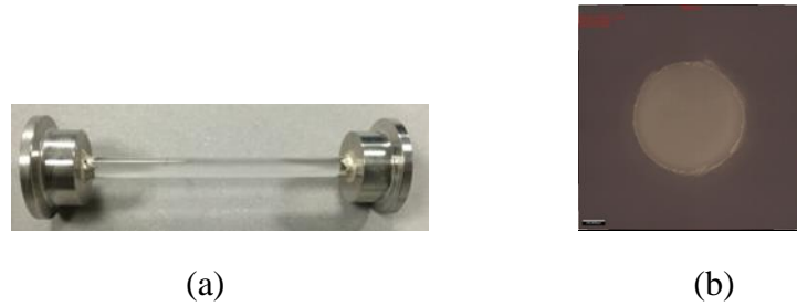
Figure 6.2: (a) Glass microtube glued to KF16 socket flanges; (b) Photo taken by the Alicona System for the measurement of the inner diameter
