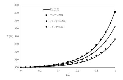
Figure 6.4: Temperature distributions along the channel obtained by the theoretical model compared with the experimental data from (Rojas-Cárdenas 2012)
