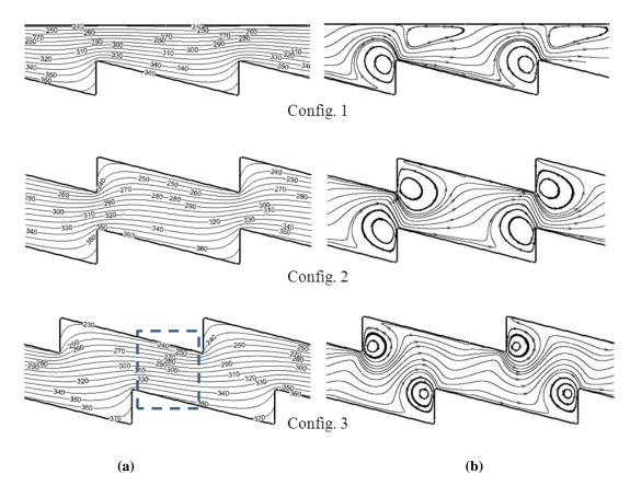
Figure 5.4: Isotherms (a) and streamlines (b) for the three configurations, with  $d = h = 1 \,\mu\text{m}$ ,  $L = 4 \,\mu\text{m}$ ,  $T_h = 375 \,\text{K}$ ,  $T_c = 225 \,\text{K}$  and  $P = 1.013 \times 10^5 \,\text{Pa}$
