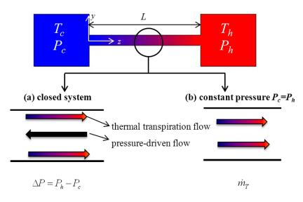
Figure 2.5: Schematic representation of transpiration flow
