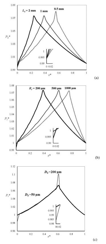
Figure 4.4: Influence of the microchannel dimensions on the dimensionless pressure  $P_2^*$  distributions along the centerline for a single-stage pump in cases 4, 5 and 6 (a), cases 1, 3 and 4 (b) and cases 1 and 2 (c).
