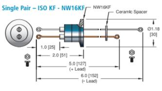
Figure 6.6: Thermocouple feedthrough
