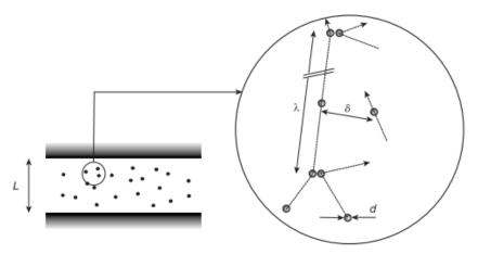
Figure 2.1: Main characteristic length scales taken into account at the molecular level (Colin 2013)
