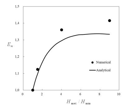
Figure 3.5: Efficiency based on the mass flowrate in tapered channels with different values of  $H_{\text{max}} / H_{\text{min}}$
