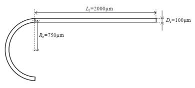
Figure 4.11: Geometry of single stage of prototype
