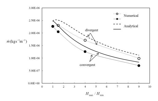
Figure 3.4: Mass flowrate generated by tapered channels with different  $H_{\text{max}} / H_{\text{min}}$ It is found that the mass flowrates generated by the divergent channels are larger than those generated by the convergent channels. Compared to the transpiration flow in a cylindrical channel, for which  $H_{\text{max}} / H_{\text{min}} = 1$ , the mass flowrate is reduced in
