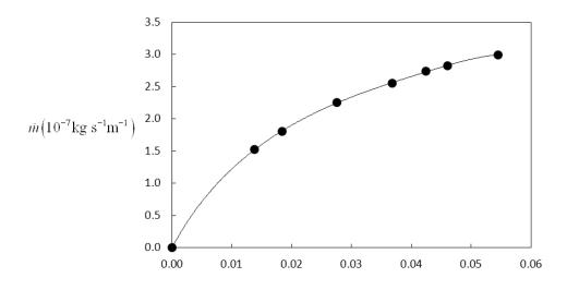
Figure 5.6: Mass flowrate per unit of width versus Knudsen number
