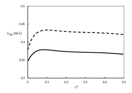
Figure 2.11: Slip velocity along the inner wall of the curved channel for isothermal flow in geometrical case 1, with  $P_A = 0.06$  Pa ,  $P_C = 0.061$  Pa , T = 300 K and  $Kn_C = 0.1$ . The dashed line does not take the term  $\partial u_n / \partial s$  from Eq. (2.3) into account but the solid
