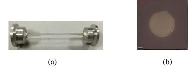
Figure 6.2: (a) Glass microtube glued to KF16 socket flanges;(b) Photo taken by the Alicona System for the measurement of the inner diameter
