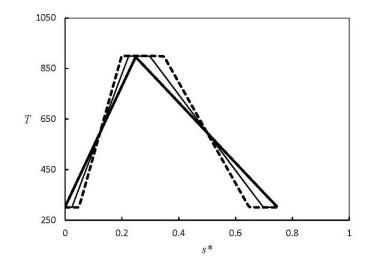
Figure 4.6: Imposed temperature distribution along the inner wall of the curved and straight parts of the channel for different sizes of the heated or cooled zones:  $L_z = 0$  (thick solid line),  $L_z = 0.1 L_s$  (thin solid line) and  $L_z = 0.2 L_s$  (dashed line).
