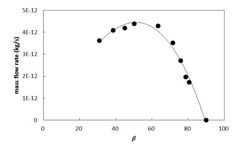
Figure 5.23: Mass flowrate for different values of the ratchet angle  $\beta$ . Kn = 0.184,  $L = 1 \ \mu m$  and  $d = h = 1 \ \mu m$
