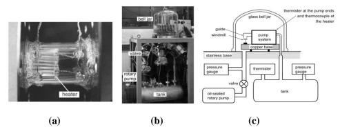
Figure 1.8 Experimental system for Knudsen pumping: (a) Real system, zoom on the pump; (b) Real system, global view; (3) explanatory diagram (Sone et al. 2003).
