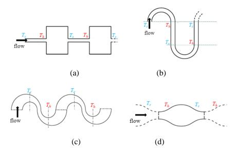
Figure 4.1: Configurations of classic Knudsen pump (a), curved-channel Knudsen pump (Aoki et al. 2009) (b), double-curved Knudsen pump (Bond et al. 2014) (c) and sinusoidal Knudsen pump (Bond et al. 2016) (d).
