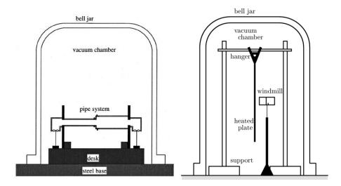
(a) One-way flow (b) Thermal edge flow Figure 1.4 Experimental apparatus for demonstration of temperature-driven flow (Sone et al. 1997, Sone et al. 2000)
