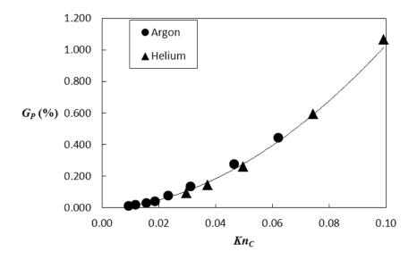
Figure 4.15: Pressure gain versus  $Kn_C$  for argon et helium for the 2-stage pump ( $T_c = 77 \text{ K}, T_h = 370 \text{ K}, P_0 = 150 \text{ Pa} \sim 1200 \text{ Pa}$ ).
