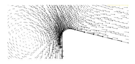
Figure 5.5: Velocity vectors near a tip of the lower ratchet surface for Config. 2
