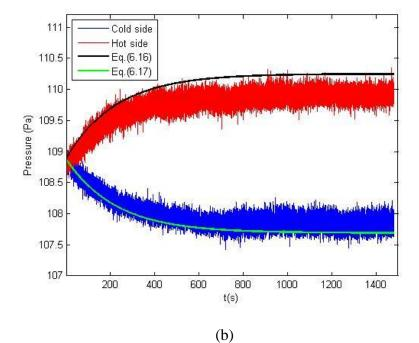
Figure 6.13: Experimental pressure variations from t = 0 to final equilibrium, compared with theoretical results of Eqs. (6.16) and (6.17).  $Kn_0 = 0.028$  (a);  $Kn_0 = 0.108$  (b)
