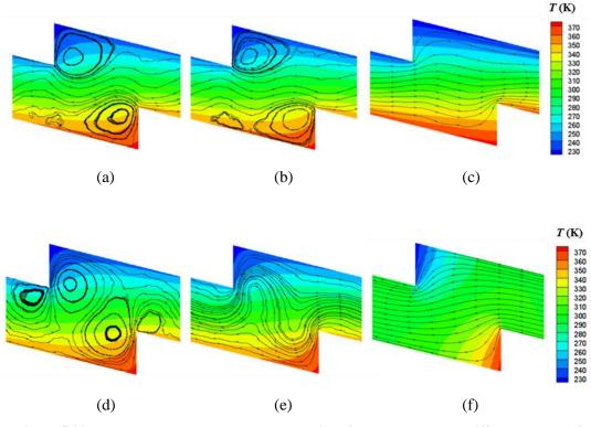
Figure 5.20: Temperature contours and streamlines for Kn = 0.184 and different values of the accommodation coefficients  $\alpha_v$  and  $\alpha_I$ :
