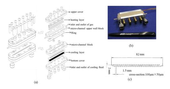
Figure 4.10: Serpentine Knudsen system fabricated by KIT. (a) sketch of the pump system; (b) photo of the final device; (c) configuration of the micro-channel
