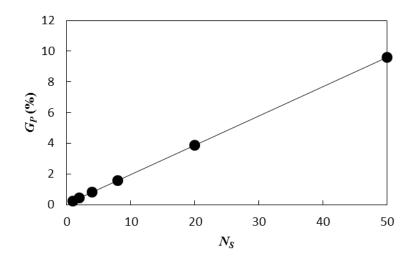
**Figure 4.12:** Pressure gain versus number of stages ( $T_c = 77 K, T_h = 370 K, P_0 = 150 Pa$
