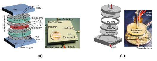
Figure 1.5 Exploded views and photos of Knudsen pumps based on:
