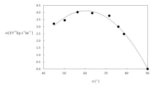
Figure 5.8: Mass flowrate per unit of width versus ratchet angle
