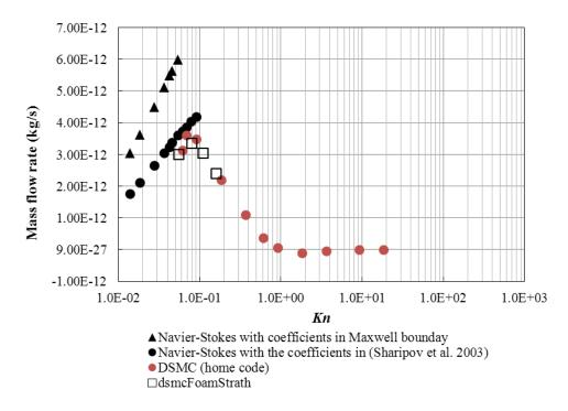
Figure 5.18: Comparison of mass flowrates obtained by DSMC and CFD
