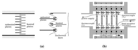
Figure 1.9 Knudsen pump based on the edge flow phenomenon: a) one stage of the pump; b) complete pump system (Sugimoto et al. 2005).
