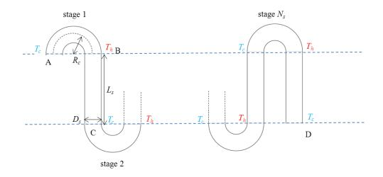
Figure 4.2: Configuration of multi-stage curved-channel pump
