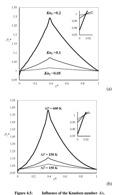
Figure 4.5: Influence of the Knudsen number  $Kn_C$ and of the temperature difference  $\Delta T = T_h - T_c$  on the dimensionless pressure  $P_2$  \* along the microchannel centerline of a single-stage micropump. a) Cases 4-a, 4-b and 4-e; b) Cases 4-b, 4-c and 4-d.
