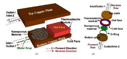
Figure 1.6Schematic of two designs of Knudsen pumpswith thermoelectric modules (Kunal et al. 2010): (a) lateral design; (b) radial design.
