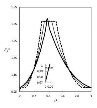
Figure 4.7: Influence of the size of the heated or cooled zones on the dimensionless pressure  $P_2$  \* along the microchannel centerline of a single-stage micropump:  $L_z = 0$  (thick solid line),  $L_z = 0.1 L_s$  (thin solid line) and  $L_z = 0.2 L_s$  (dashed line).
