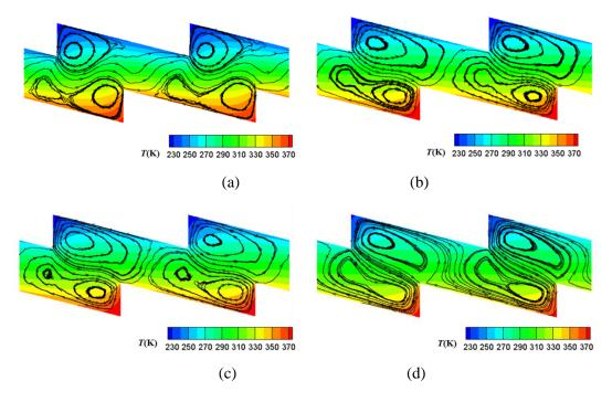
Figure 5.19: Streamlines and iso-contours of temperature for different values of the Knudsen number: a) Kn = 0.184, b) Kn = 0.613, c) Kn = 0.920 and d) Kn = 1.840
