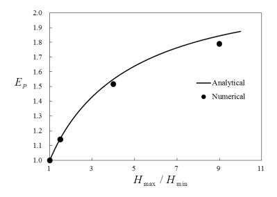
Figure 3.7:Efficiency on the pressure difference generated by tapered<br/>channels for different values of  $H_{max} / H_{min}$
