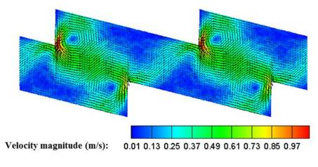
Figure 5.14: Velocity vectors and iso-contours of velocity magnitude for the reference case at Kn = 0.16
