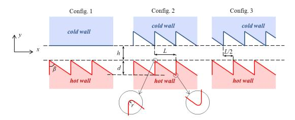
Figure 5.2: Three analyzed configurations and geometric parameters
