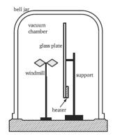
Figure 1.3 Experimental apparatus for demonstration of thermal transpiration flow (Sone 1991)
