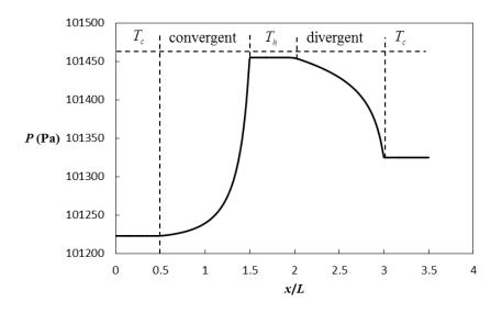
Figure 3.11: Pressure distribution along the tapered-channel pump
