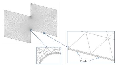
Figure 5.3: Mesh 1 and details at the wall
