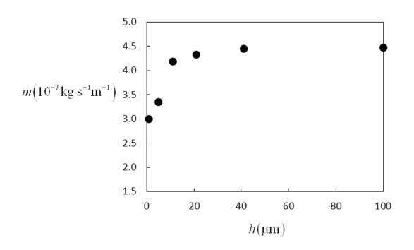
Figure 5.9: Mass flowrate versus distance between channel walls
