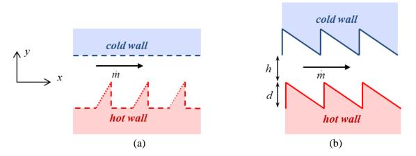
Figure 5.1: Two ratchet designs analyzed by (a) Donkov et al. (Donkov et al. 2011) and (b) Würger (Würger 2011). In (a), diffusive walls are represented by dashed lines and specular walls by dotted lines.
