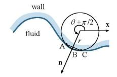
Figure 2.7: Osculating circle at the wall for determination of  $\theta$  derivatives.
