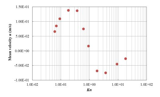
Figure 5.17: Mean velocity versus Knudsen number
