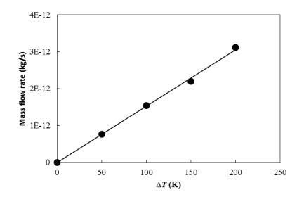
Figure 5.15: Mass flowrate for different temperature differences
