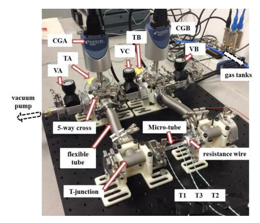
Figure 6.3: Photo of the experimental set-up
