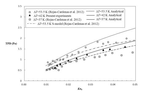
Figure 6.9: Thermomolecular pressure difference in the slip flow regime compared with analytical and numerical results.
