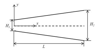
Figure 3.2: Schematic of a tapered channel
