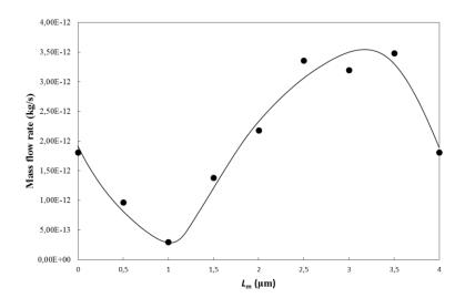
Figure 5.21: Mass flow rate versus misalignment distance  $L_m$ ;
