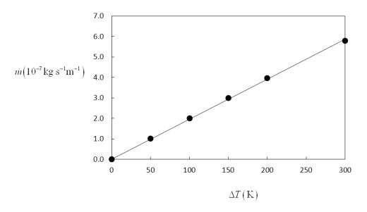
Figure 5.7: Mass flowrate per unit of width versus temperature difference
