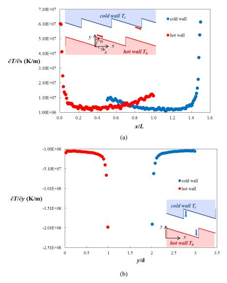
Figure 5.13: Tangential temperature gradients in the gas close to the ratchet surfaces for the reference case at Kn = 0.184 along the a) inclined walls, b) vertical walls
