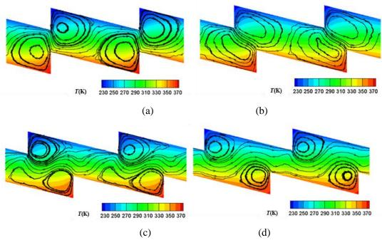
Figure 5.22: Temperature iso-contours and streamlines for different misalignment distances; Kn = 0.184, L = 1 μm and d = h = 1 μm.
