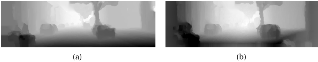
Figure 3.3: Two depth maps computed using two pairs of images that shares the same first image. (a) The image pair are shifted horizontally (stereo pair); (b) The image pair are obtained with dominant forward motion (Epipole near the center, borders problem).
