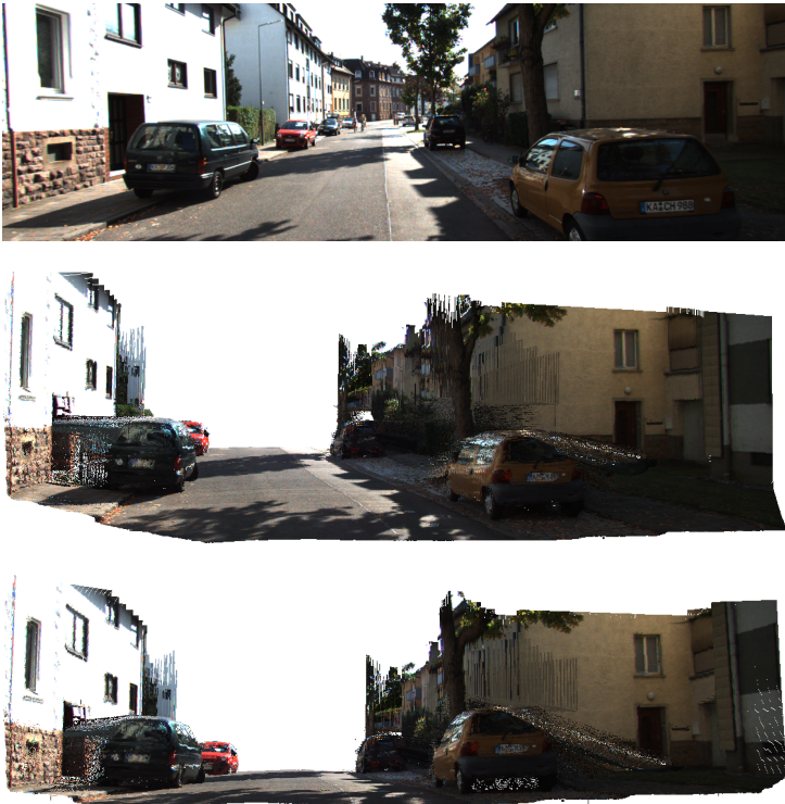
Figure 5.7: Original frame from the sequence 95 and a Dense 3D model obtained using the proposed method from several view points.
