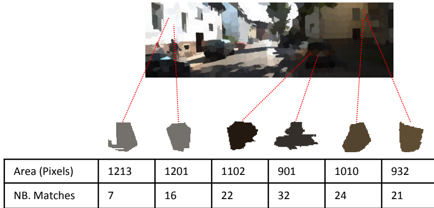
Figure 4.5: Example of superpixels obtained using original SLIC method [Achanta 2012].
