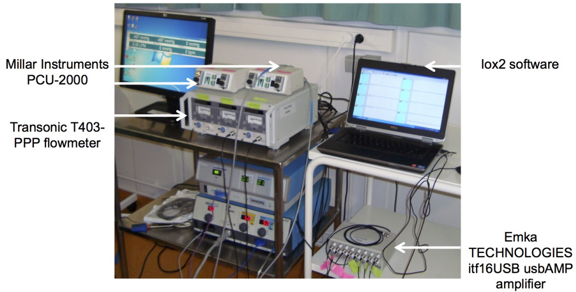
Figure 2.6: Recording installation for pressures, Millar Instruments PCU-2000 and for flows, Transonic T403-PPP flowmeter. emka TECHNOLOGIES itf16USB usbAMP amplifier and the computer with iox2 software.
