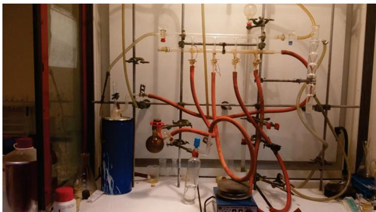
Figure 7.1 – Vacuum-Schlenk system with Schlenk glassware to work under inert atmosphere.
