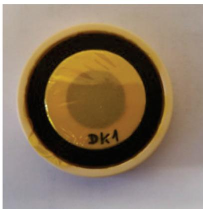
Figure 7.4 – X-ray sample holder equipped with a kapton film.
