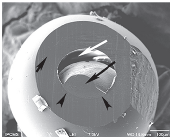
Figure 13 SEM micrograph of a core-shell polymeric microparticle.
