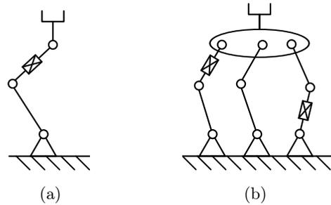
Figure 1.1 – Open and closed kinematic chains.
