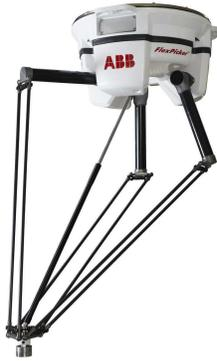
Figure 1.4 – The Delta *IRB 360 FlexPicker* by ABB®.
