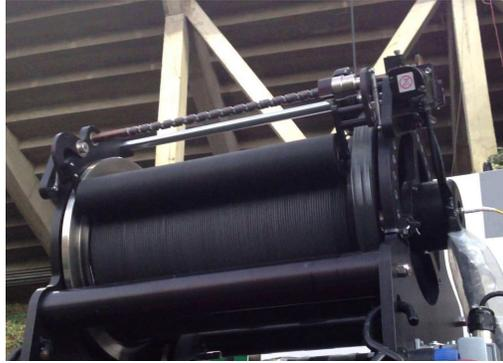
(b) A SkyCam motorized reel [SkyCam 2015].
