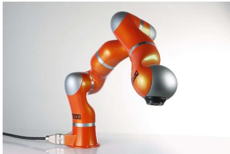
Figure 1.2 – The Kuka<sup>®</sup> 7-dof robotic arm.
