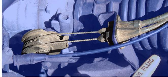
Figure 1.7 – Bowden cables controlling an automobile throttle [Ehardt 2015].
