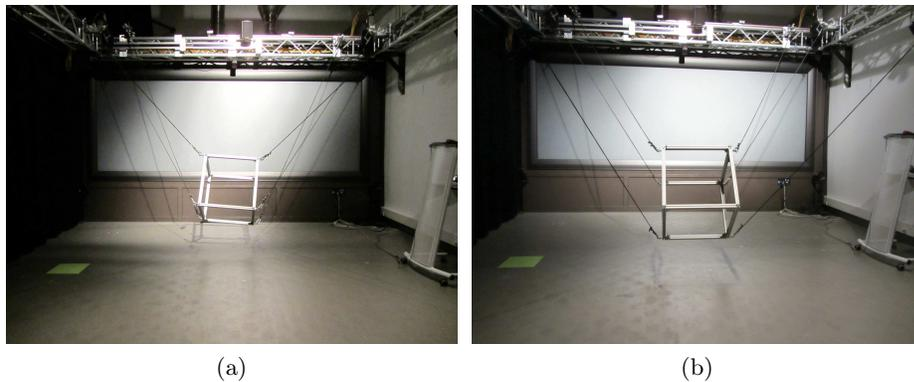
Figure 4.6 – Validation of Test 3 on the large scale robot MARIONET-VR: (a) configuration No. 1 with 6 cables in tension; (b) configuration No. 3 with 6 cables in tension.
