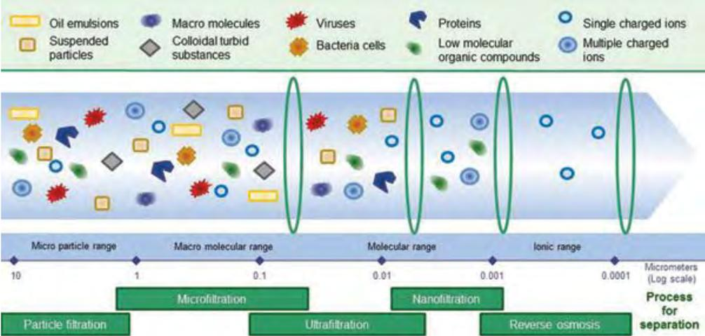
Figure 1.1: Separation ranges for various membrane processes
