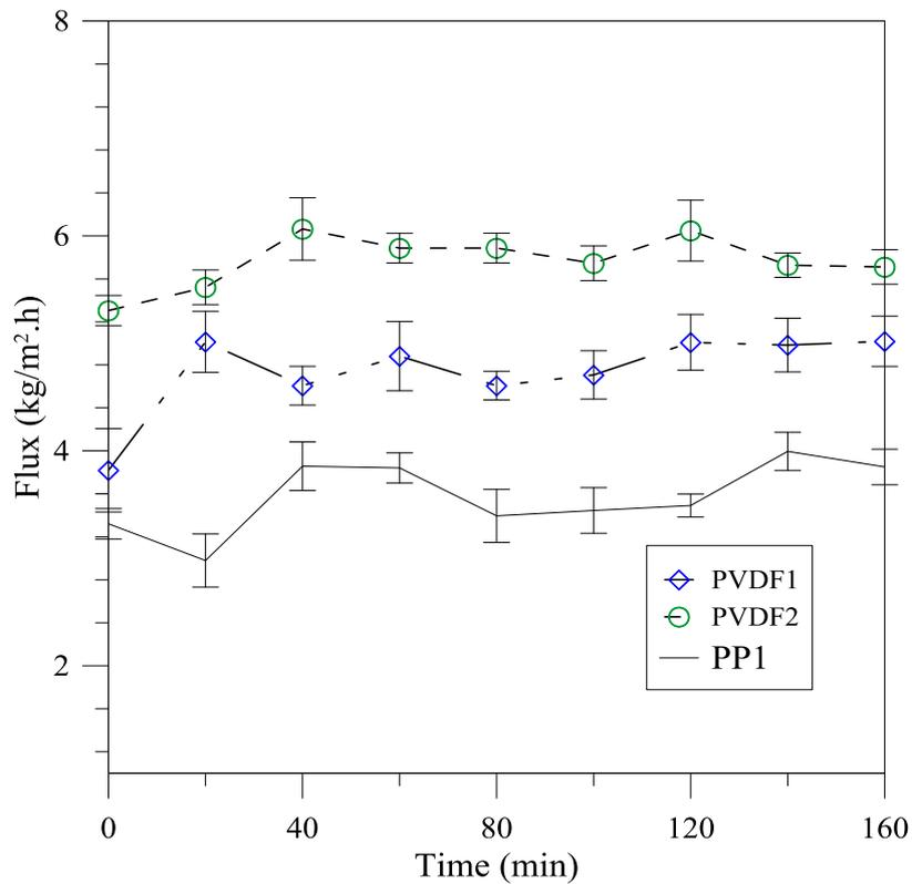
Figure 6.15: Flux obtained for PP1, PVDF1 and PVDF2 membranes after 8 weeks of storage
