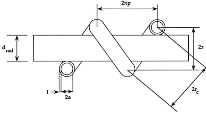
Figure 5.1: A tube helically wrapped around a rod
