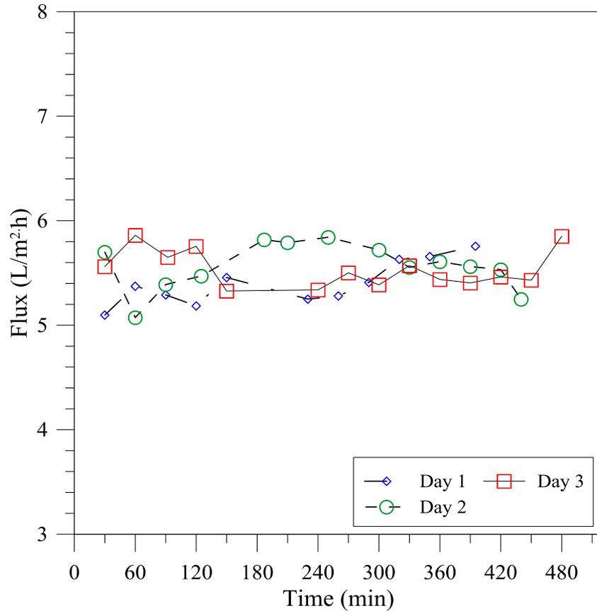
Figure 7.8: Flux obtained for MBR effluent as function of time by using PP membrane
