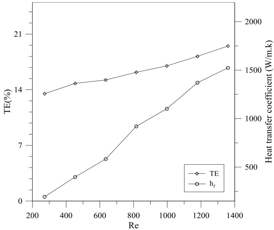
Figure 4.5: Effect of Reynolds number on thermal efficiency and heat transfer coefficient
