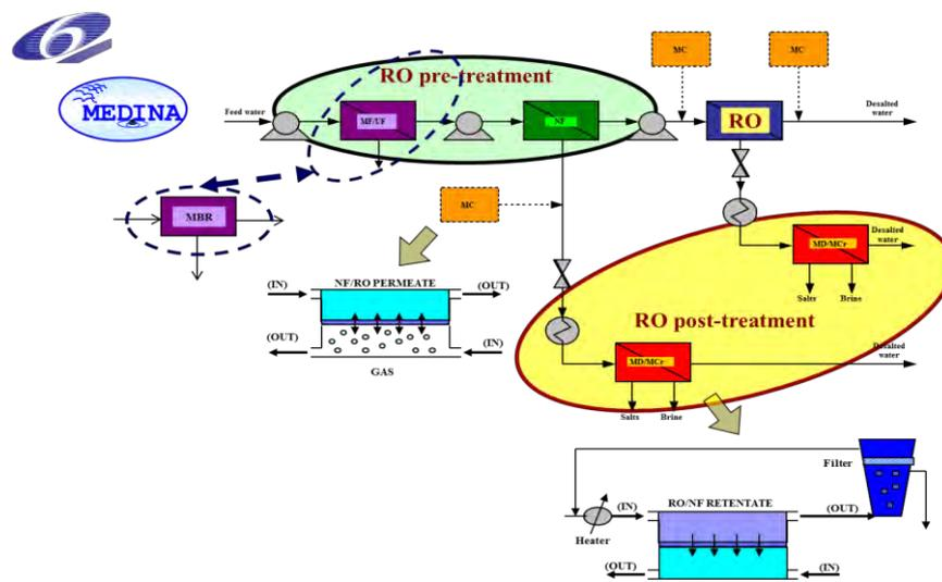
Figure 1.2: Integrated membrane systems for desalination proposed in MEDINA project [5]
