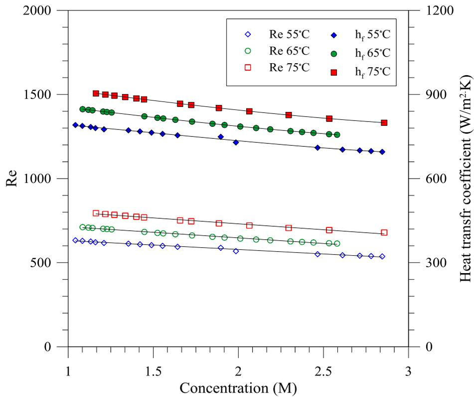
Figure 4.13: Dependence of heat transfer coefficient and Re on feed solution concentration
