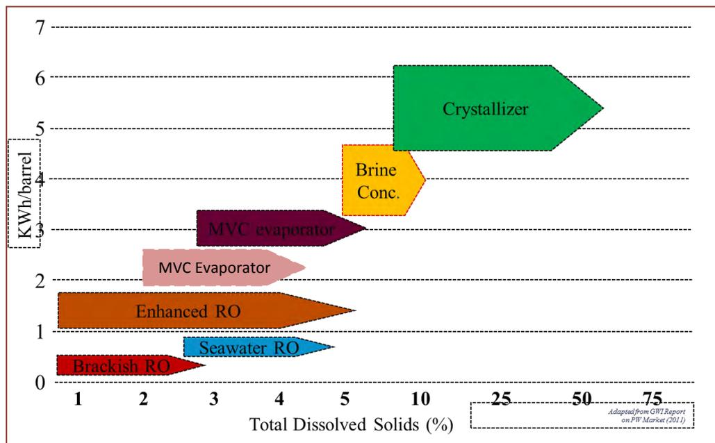
Figure 6.3: A comparison of desalination technologies on the basis of energy consumption, feed concentration and maximum achievable salinity level
