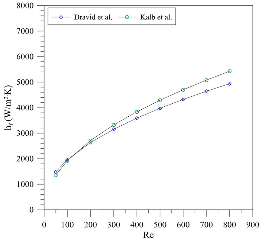
Figure 5.8: Effect of  $Re$  on heat transfer coefficient according to various correlations
