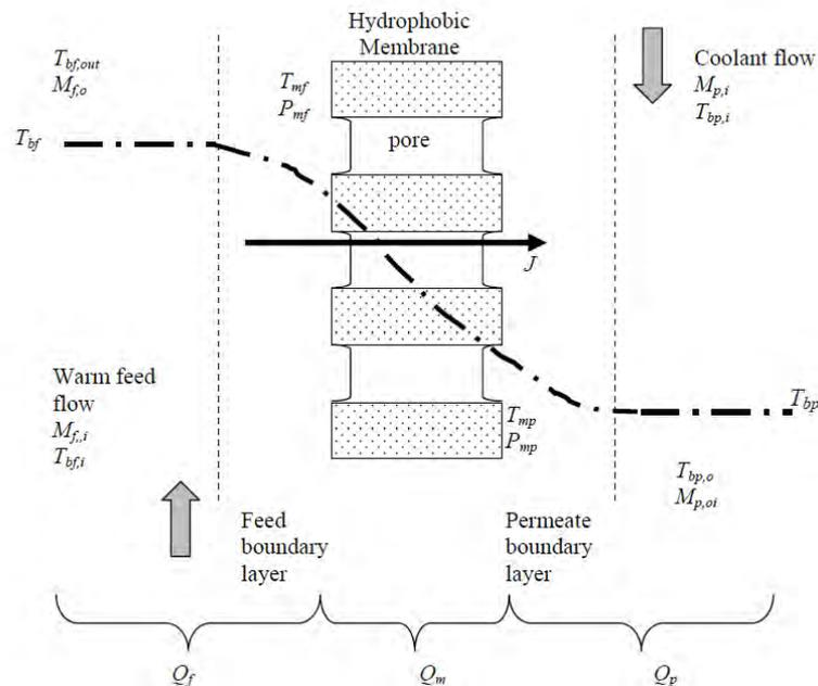
Figure 1.4: Illustration of heat transfer and thermal polarization in MD process
