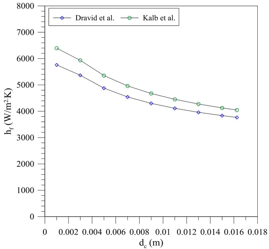
Figure 5.9: Effect of coil diameter on feed side heat transfer coefficient at  $Re=444$  and pitch of 4mm
