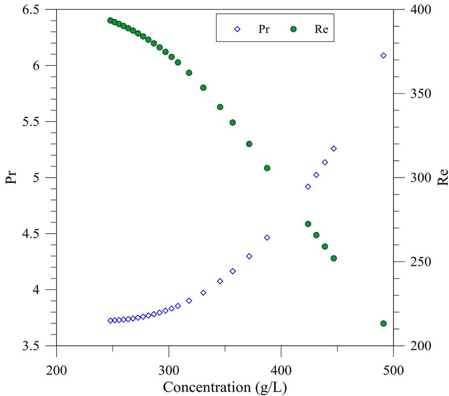
Figure 7.5: Effect of solution concentration on Pr and Re
