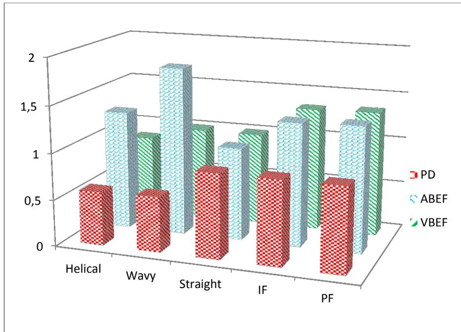
Figure 5.20: Packing density (PD), area based enhancement factor (ABEF) and volume based enhancement factor (VBEF) for different configurations and flow patterns
