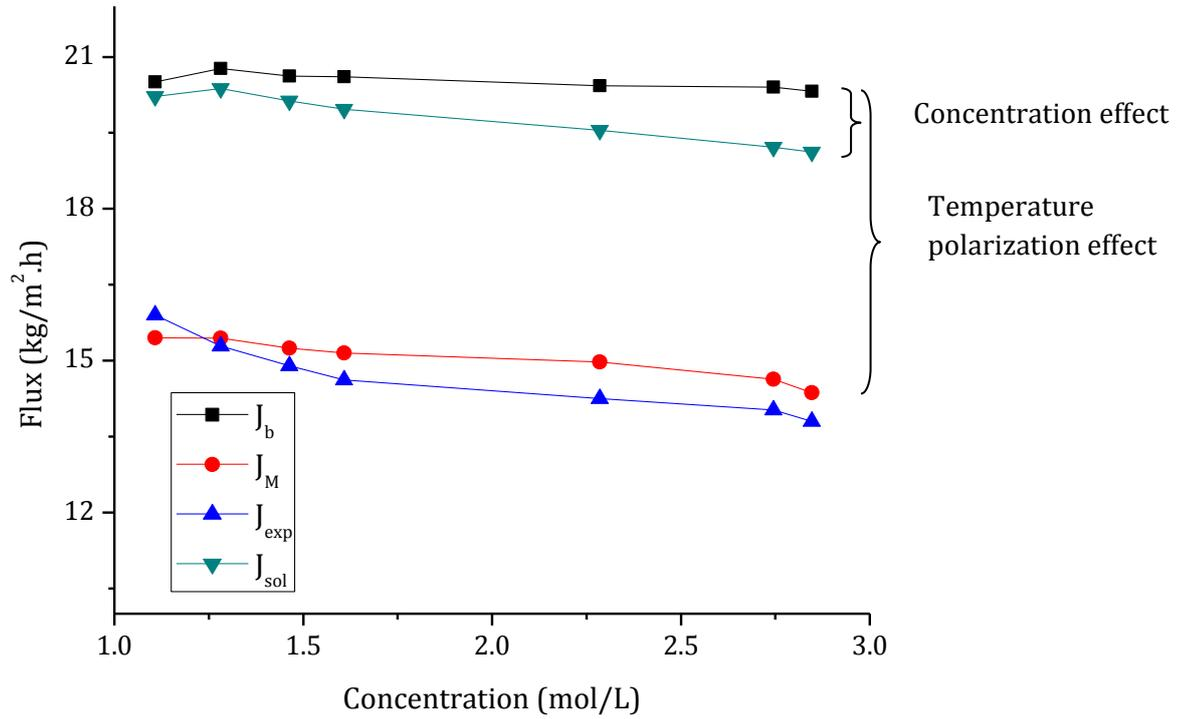
Figure 4.11: Flux calculated on the basis of different considerations and the effect of feed solution concentration and temperature polarization on reduction in flux.  $J_b$ ,  $J_M$ ,  $J_{sol}$  and  $J_{exp}$  represent the flux calculated on the basis of bulk temperatures, temperature at the membrane surface, on the basis of bulk temperatures combined with solution concentration effects and experimental flux, respectively. Feed inlet temperature was 77°C
