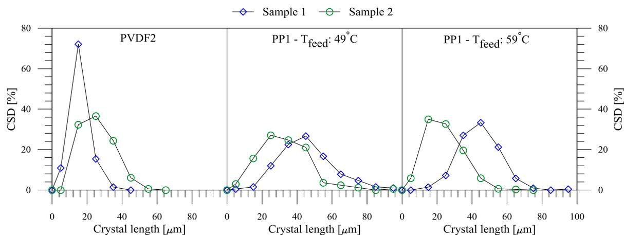
Figure 6.18: Crystal size distribution (CSD) achieved during crystallization of produced water (a) PVDF2, (b) PP1- $T_{\text{feed}}$ : 49°C, (c) PP1- $T_{\text{feed}}$ : 59°C.
