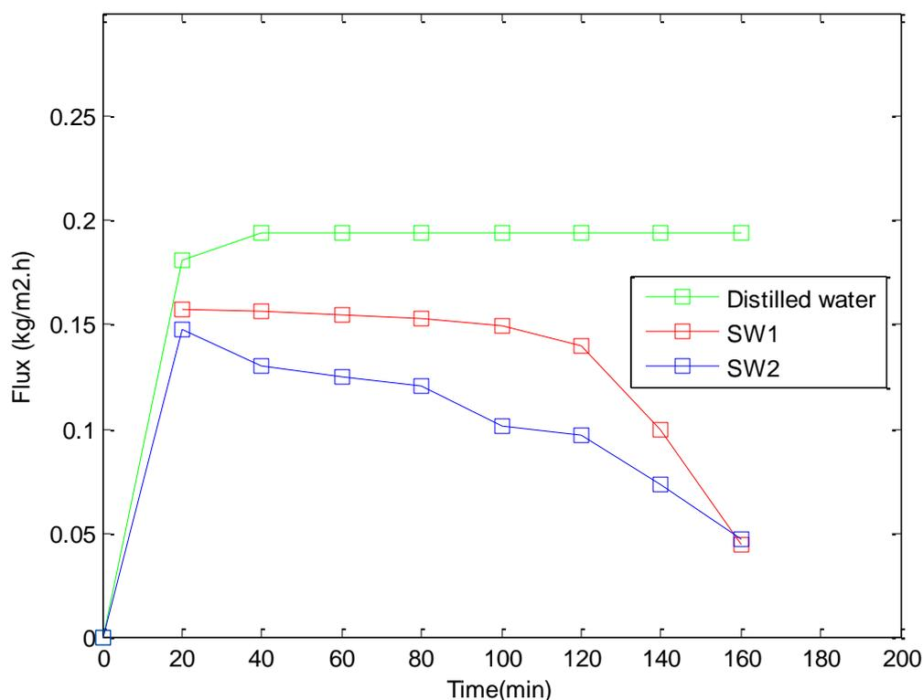
Figure 6.14: Flux obtained by using ceramic membranes. SW1 and SW2 indicate the flux obtained with new membranes and washed membranes after wetting, respectively
