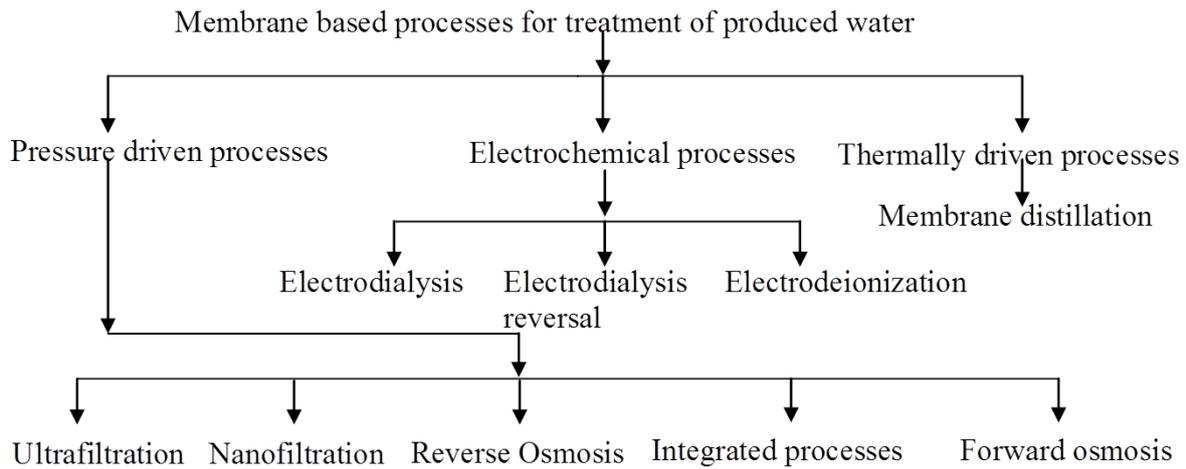
*Figure 6.2: Schematic of membrane processes for produced water treatment*
