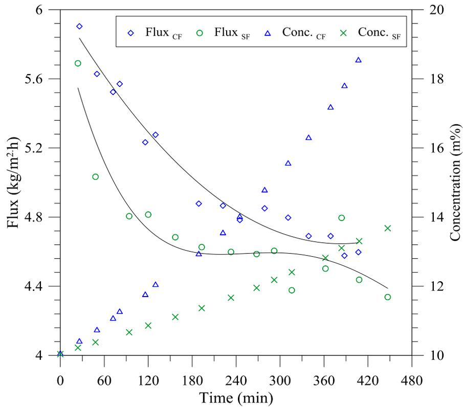
Figure 5.15: Flux achieved for straight (FS) and helical coiled (FC) modules with whey solution as feed
