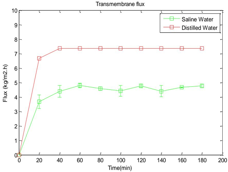
Figure 6.8: Trans-membrane flux obtained by using lab-made PVDF1 based hollow fiber membrane.
