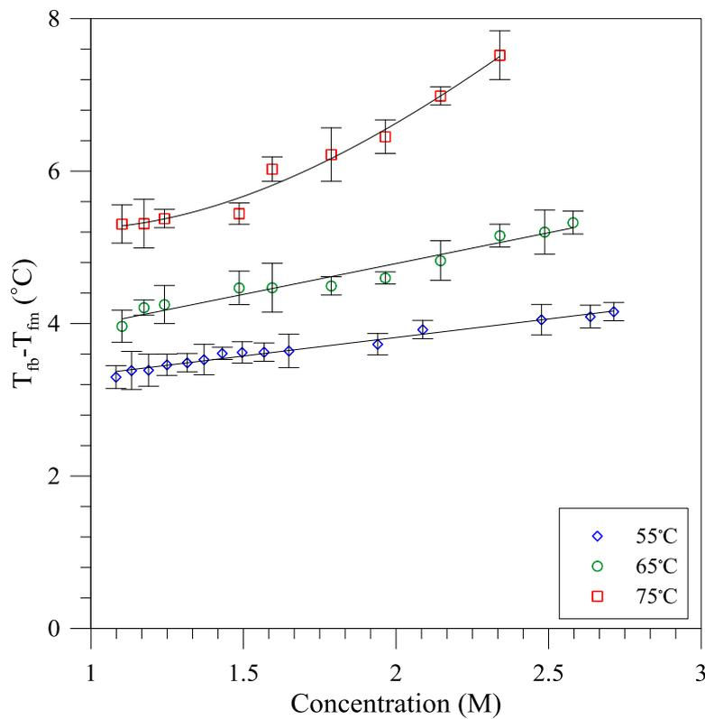
Figure 4.14: Temperature gradient between bulk and membrane surface on feed side as function of feed solution concentration at different temperatures
