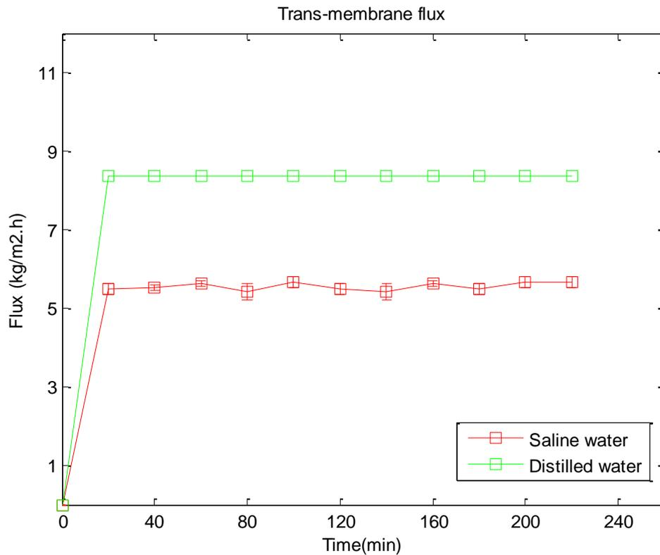
Figure 6.9: Flux obtained by using fiber type PVDF2
