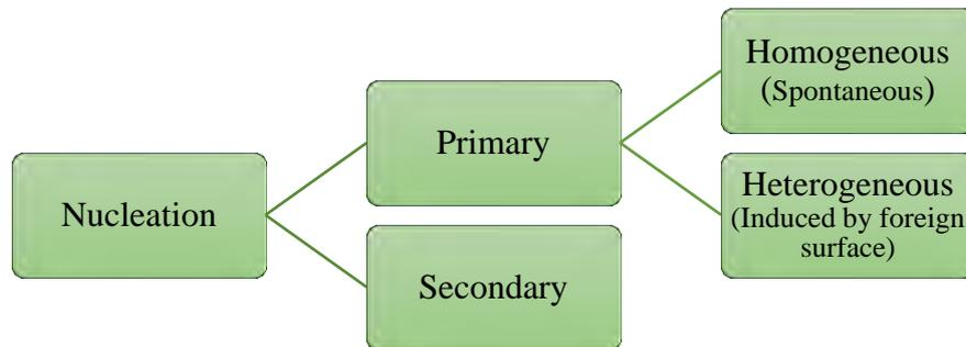
Figure 6.4: Principles of nucleation theory Adapted from [28]
