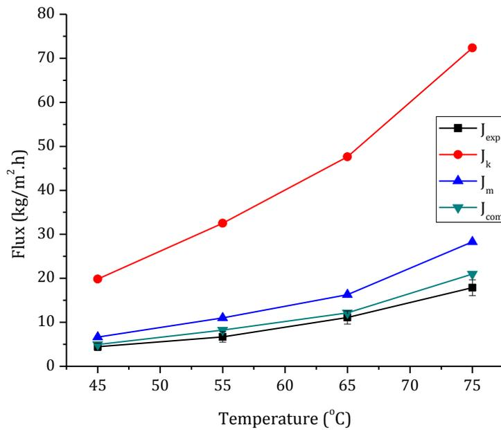
Figure 4.7: Effect of feed inlet temperature on trans-membrane flux.  $J_{exp}$ ,  $J_k$ ,  $J_m$  and  $J_{com}$  represent the experimental flux and that calculated on the basis of Knudsen diffusion model, molecular diffusion model and combined Knudsen and molecular diffusion models, respectively.
