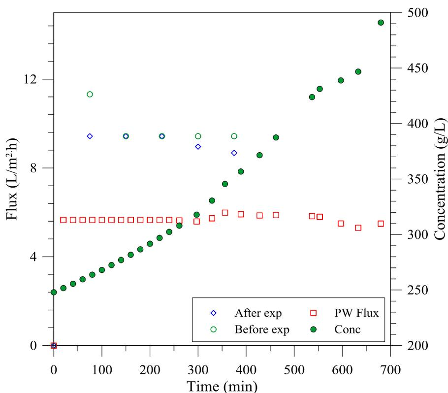
Figure 7.15: Flux for produced water during crystallization and the corresponding concentration along with pure water flux before and after crystallization.
