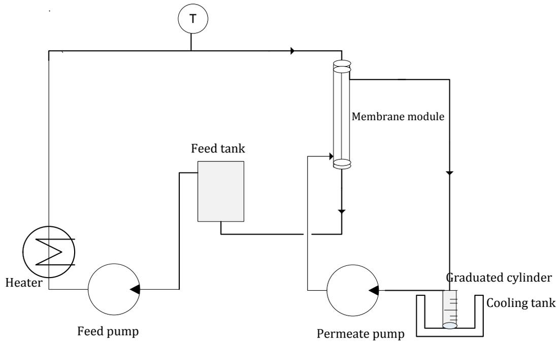
Figure 7.6: Schematic diagram of membrane distillation set-up used
