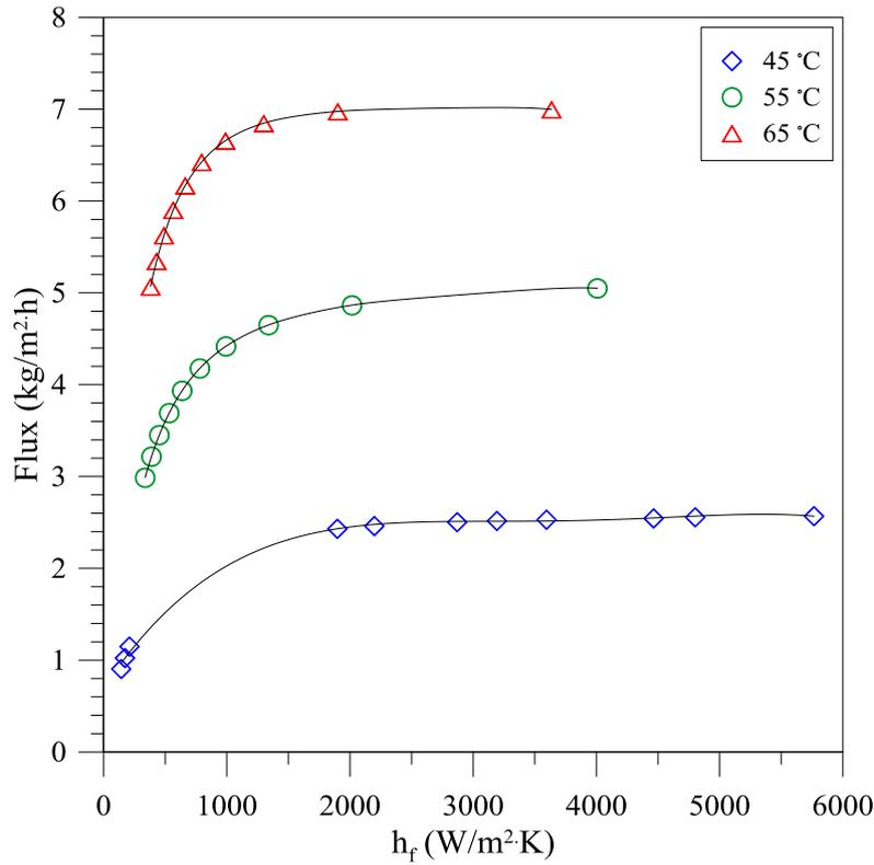
Figure 5.5: Variation of flux with heat transfer coefficient
