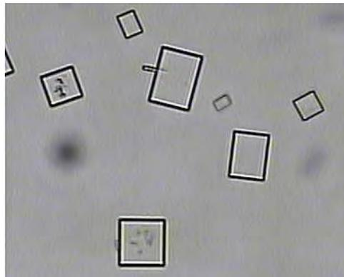
Figure 6.19: Sodium chloride precipitated from produced water.
