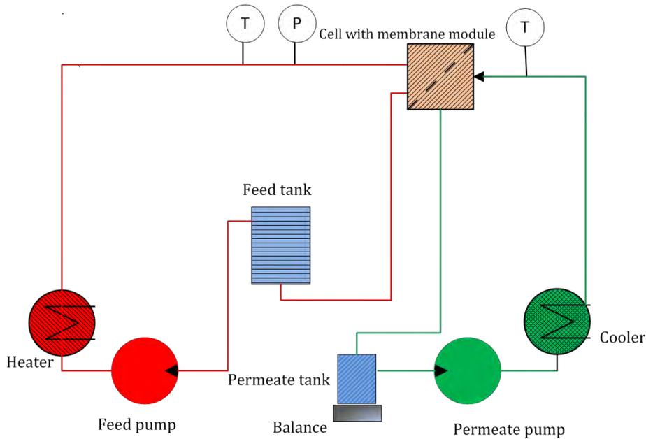
Figure 4.2: Set-up used in the experimentation
