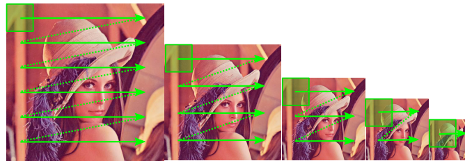
Figure 2.5: Multiscale processing via a series of lower resolution images forming an image pyramid. For faces to be detected, their dimensions need to be similar to the detector size. In order to detect faces at any distance from the camera, the 20x20 pixel detection window is scanned over all possible image pyramid locations.
