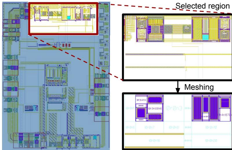
Figure 6.22: Test chip fabricated by *ams AG* ( $0.35\mu\text{m}$  HV-CMOS), and the chosen test case
