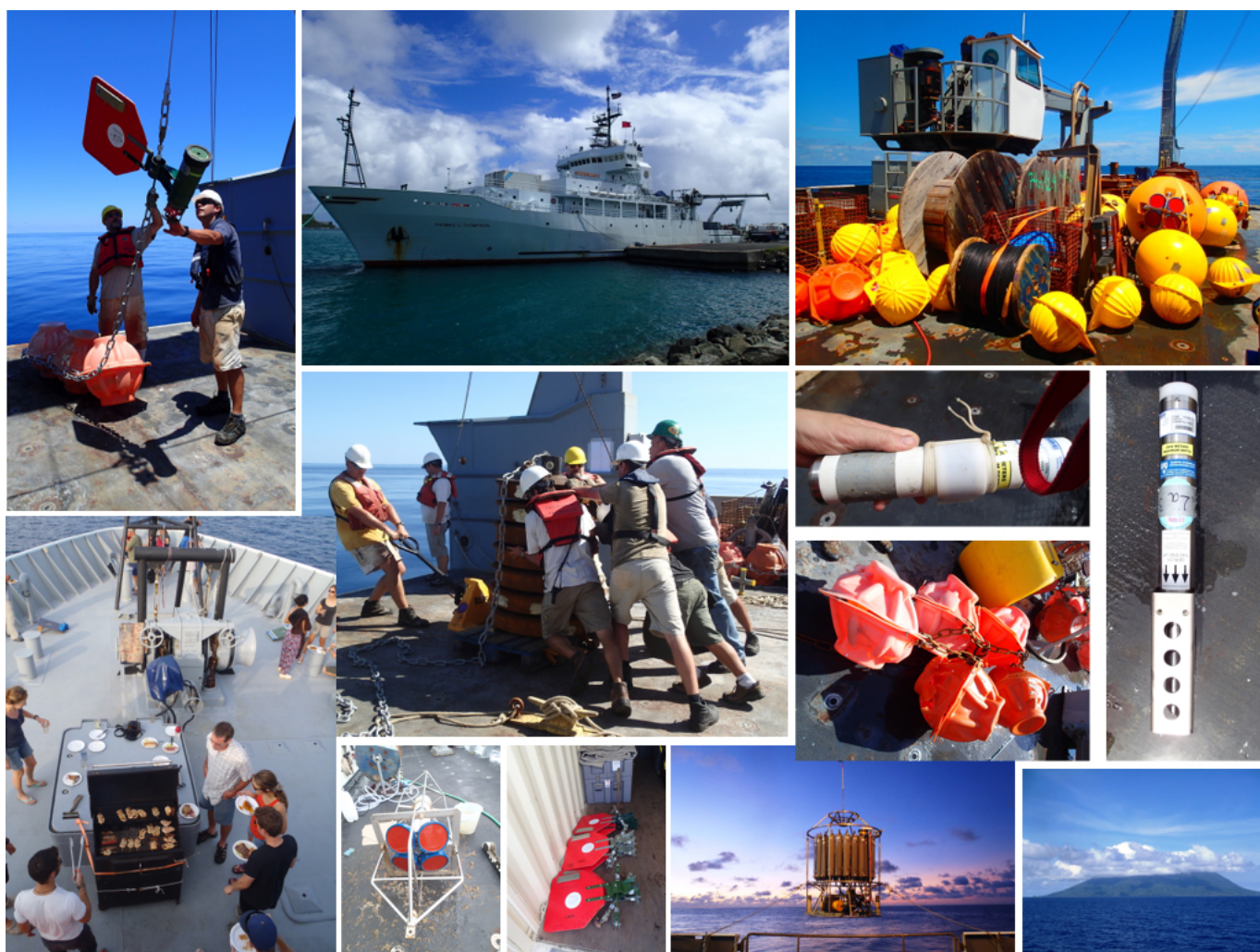
Figure 2.2 – Pictures during the MoorSPICE cruise, on the R/V Thomas G. Thompson from 28 February to 31 March 2014. Subsurface mooring instruments including T-S sensors, up-and down-looking ADCPs (right) and current meters (bottom), were firstly recovered and then deployed (upper left) at the narrow exit passages of the Solomon Sea. CTD measurements and bottle samples were carried out using a rosette system (bottom) along the cruise track (photos: C. Germaineaud and S. Cravatte).
