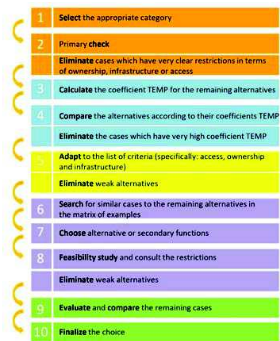
Figure 23: Schematic process for changing a mono-functional space to a multifunctional one (Ghafouri, 2016)
