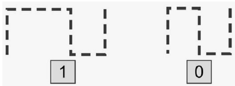
Figure 2.10: Pulse-Interval Encoding (PIE) Baseband Symbols
