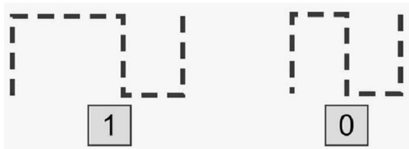
Figure 2.10: Pulse-Interval Encoding (PIE) Baseband Symbols
