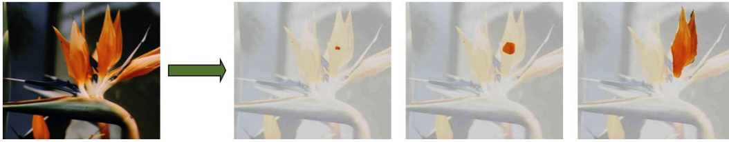
Figure 3.5: From left to right: original image and segmentation resulting from an iterative adding of pixels belonging to the neighbourhood of an initial seed [98].
